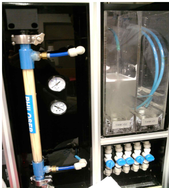
Fig. 32. Fractionation of the boiled abalone by-products by ultra-filtration membrane system with various UF membranes of MWCO 100 kDa, 10 kDa, and 1 kDa
