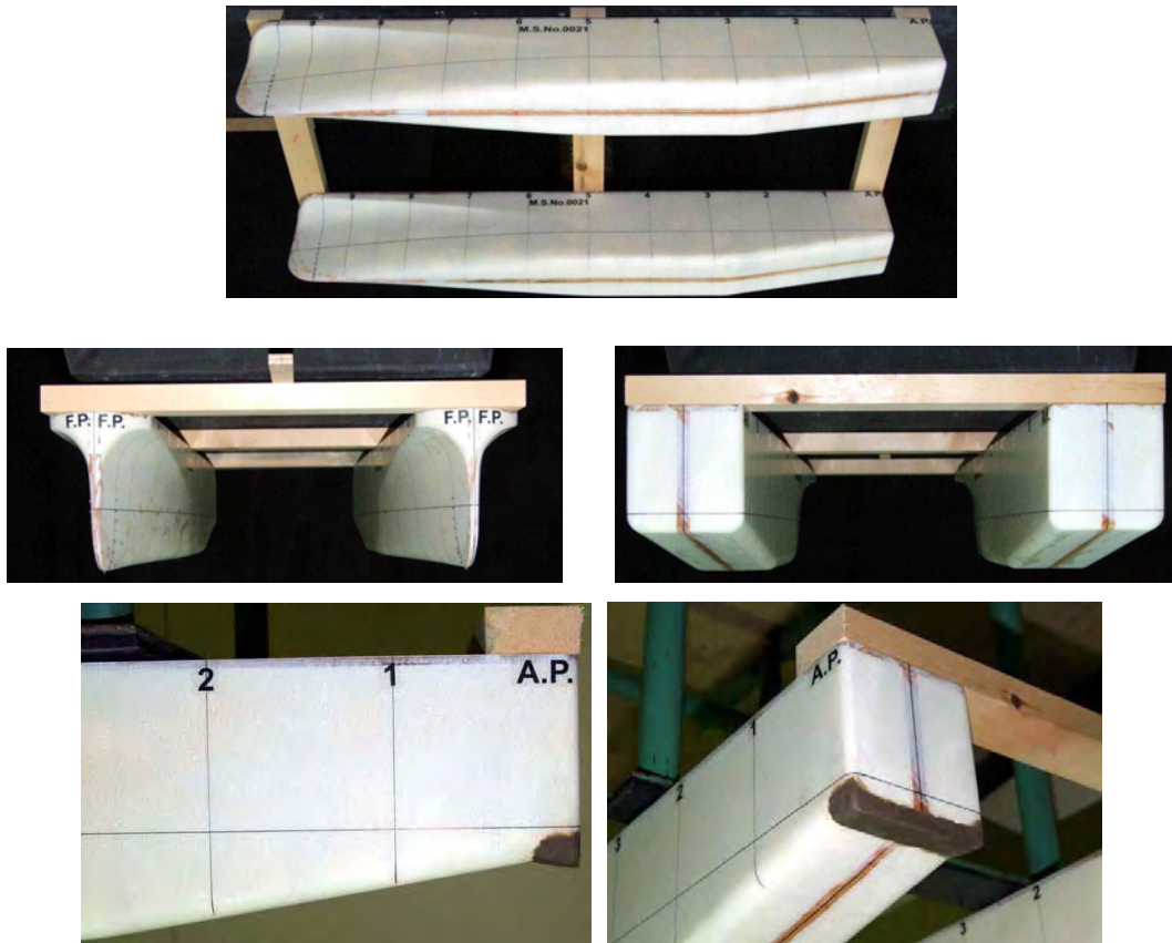
Fig. 5.2.2 Test model of L_{pp}=6.5\text{m} boat
