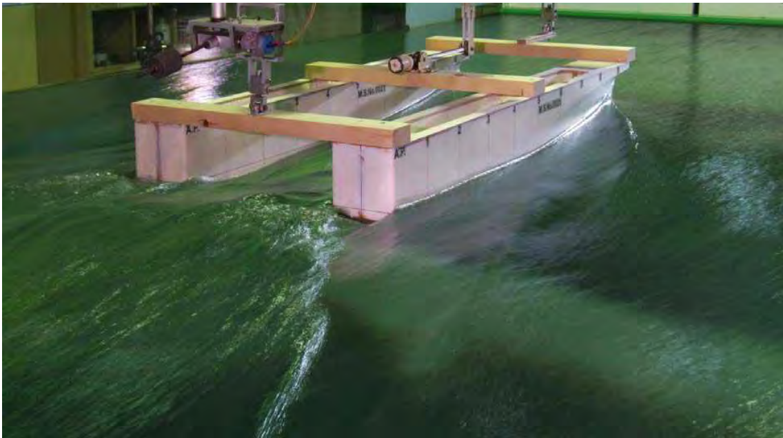
Fig. 5.2.14 Flow patterns, W/Trim tab, V=7.0 knots
