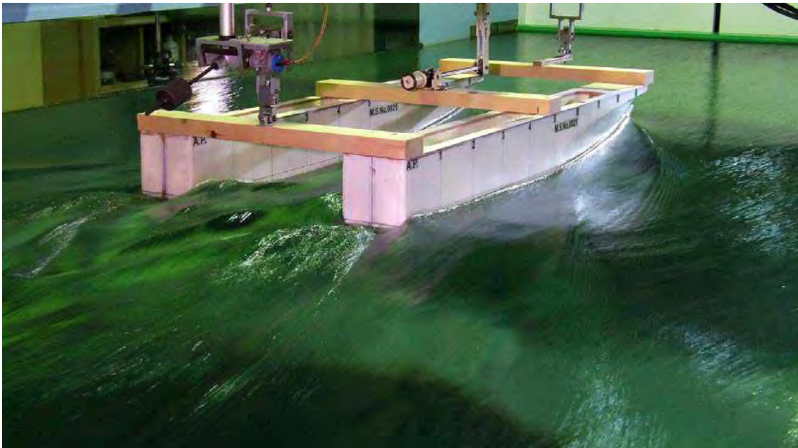
Fig. 5.2.13 Flow patterns, W/Trim tab, V=6.0 knots
