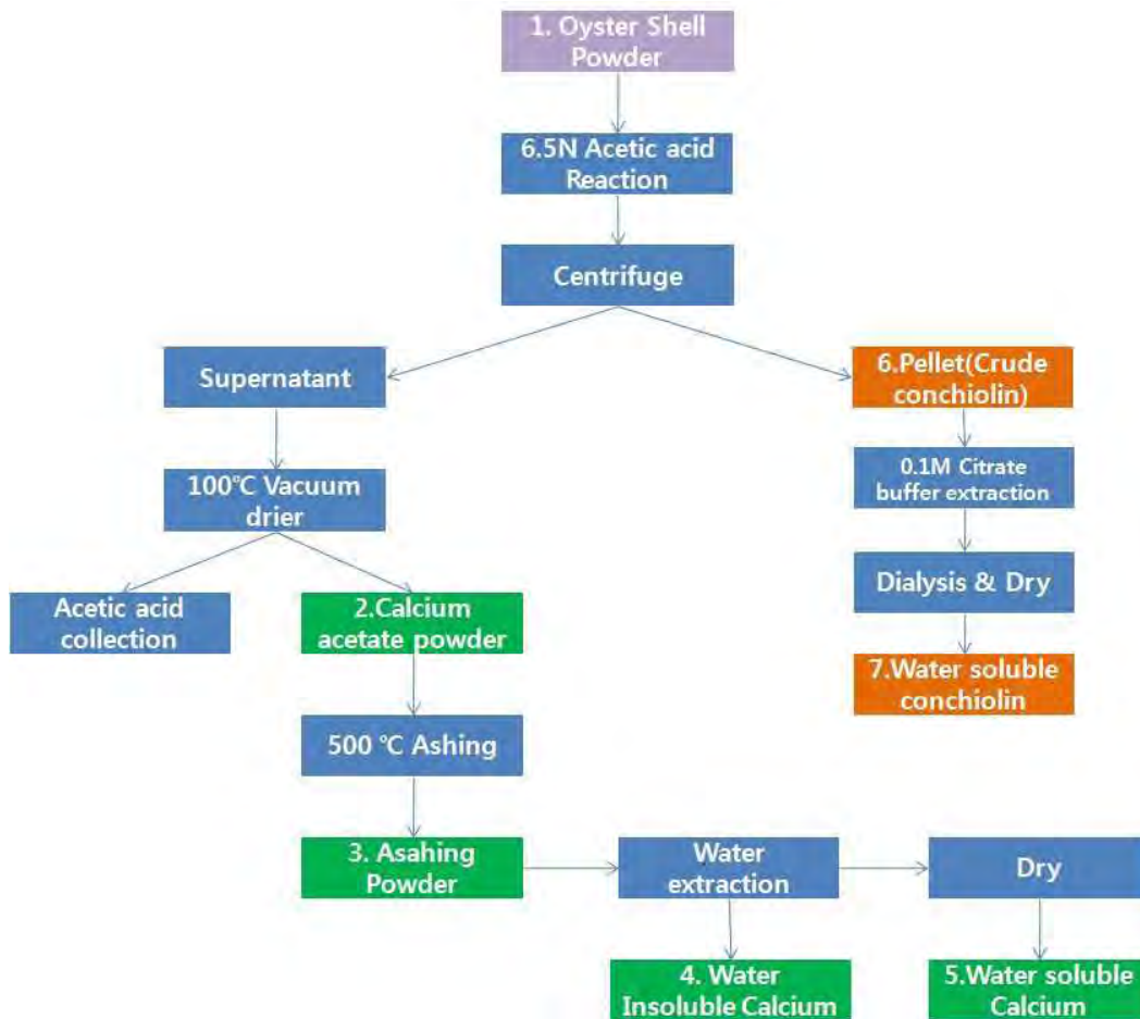
Fig. 77. Collection diagram of calcium and conchiolin from oyster shell powder.
