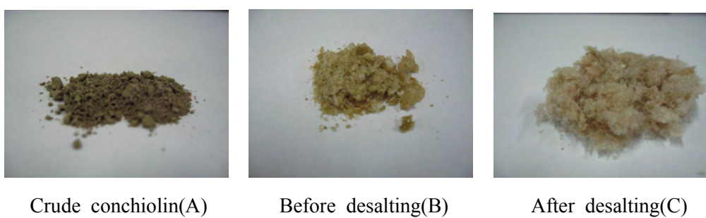
Fig. 57. Extracted conchiolins on each phase of the process.
