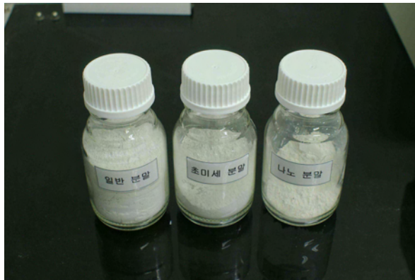
Fig. 12. Comparative photograph of normal, hyperfine and nano-scale powder.
