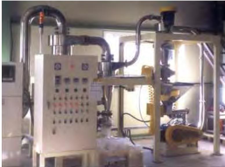
Fig. 1. Air mill equipment (Model: HTM100, Powder Technology & System Engineering Co.,Korea)
