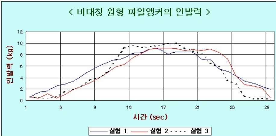
Figure 2-5. Pulling force for unsymmetric circular pile anchor.
