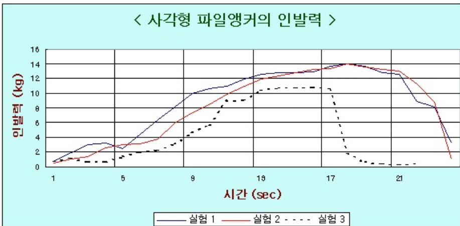
Figure 2-6. Pulling force for square pile anchor.
