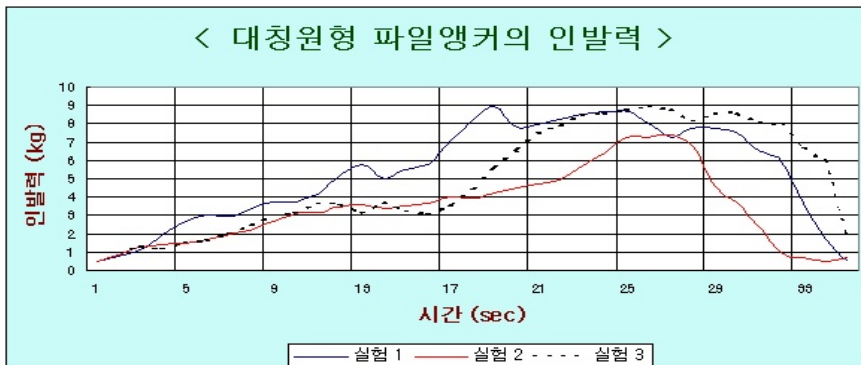
Figure 2-4. Pulling force for symmetric circular pile anchor.
