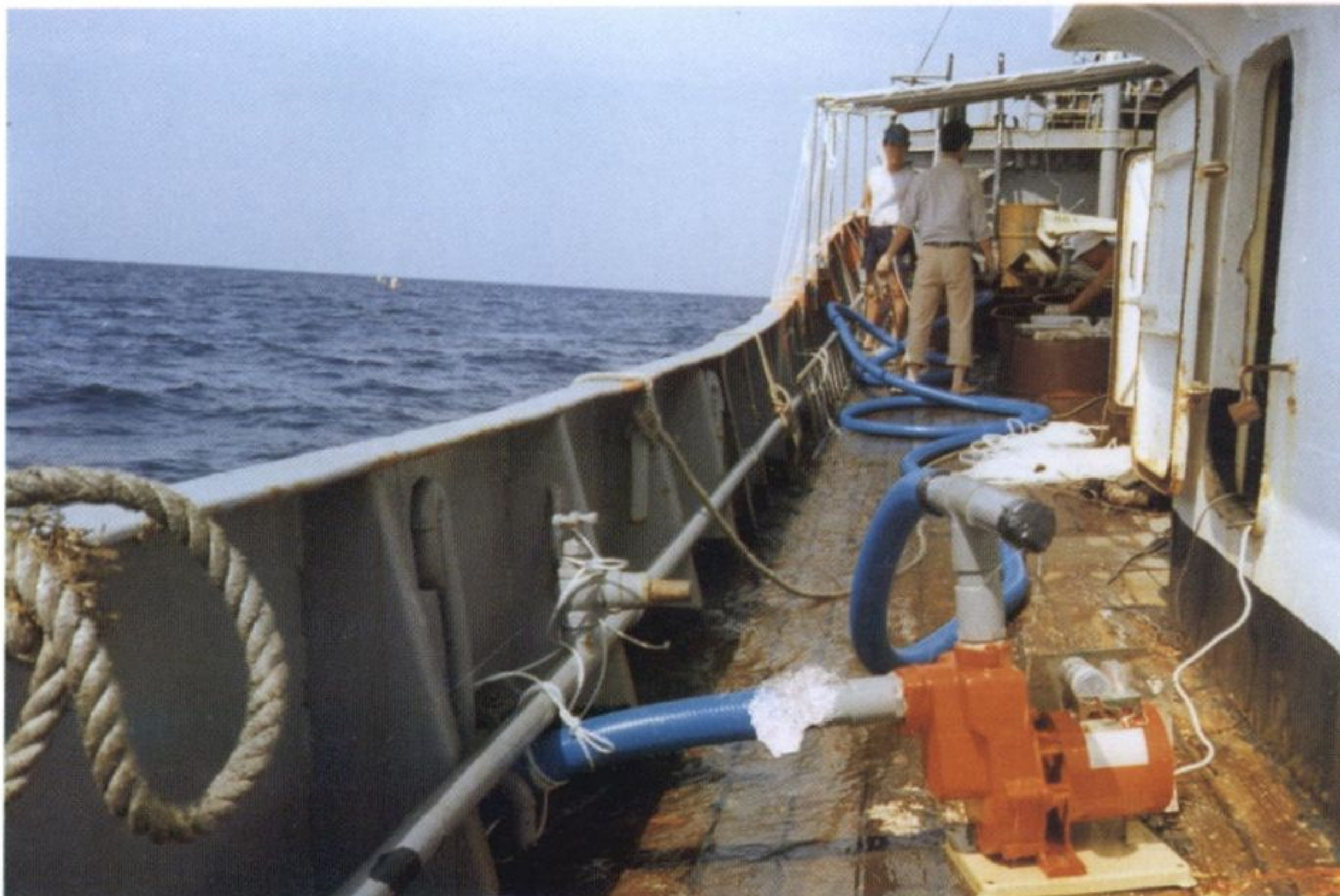
여름철 본양성 이식시 피해를 줄이기 위해 수심 20m부근의 저층저온해수 양수. For minimizing of thermal damage at transplantation of scallops for hanging culture in summer season, the lower temperature sea water from 20m depth were pumped.
