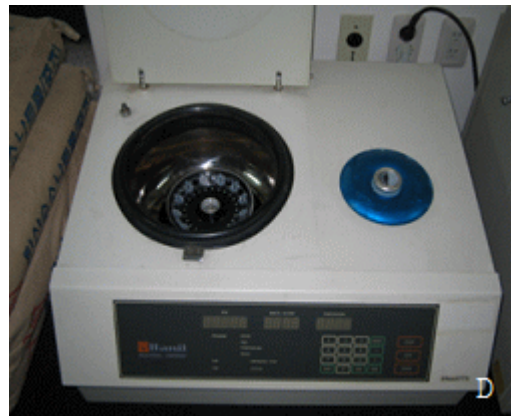
Photo 7. Cryoprotectants removal. The suspension was transferred into a tube(A and B) and it was gradually diluted by ice-chilled seawater(C). and the centrifugal separation was performed for supernatant removal(D).
