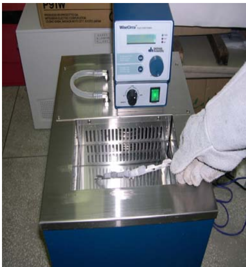
Photo 6. Thawing in a water bath at 40°C(left) and put into an ice bath(right).
