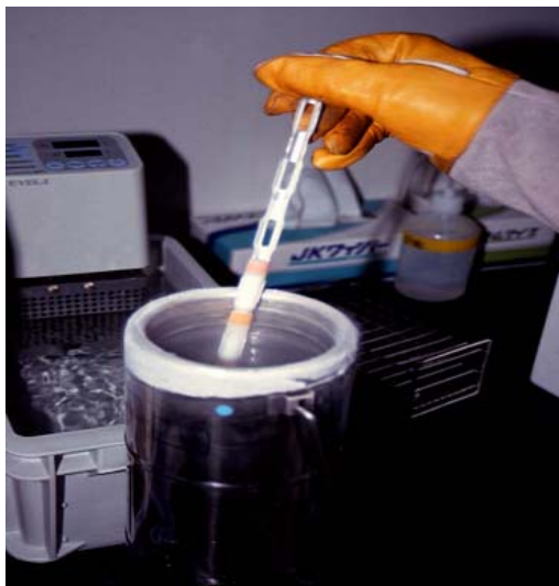
Photo 4. Rapid cooling in LN. Immersing rapidly a holder with vials into LN.
