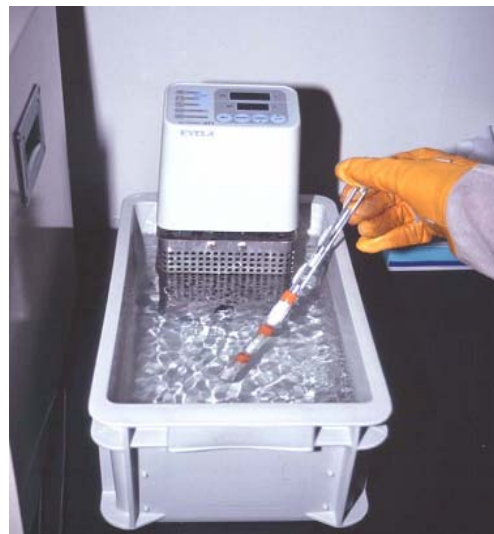
Photo 6. Thawing in a water bath at 40°C(left) and put into an ice bath(right).
