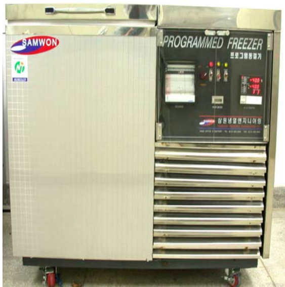
Photo 3. A programmable freezer for prefreezing. Slow cooling to -40^{\circ}\text{C} at a speed of 1^{\circ}\text{C} / \text{min} .
