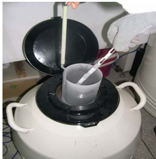
Photo 4. Rapid cooling in LN. Immersing rapidly a holder with vials into LN.
