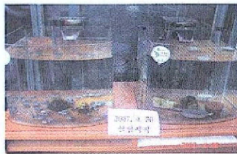
Fig. 5-16. Observation beginning of moss variation to the improved sinker and the lead sinker
