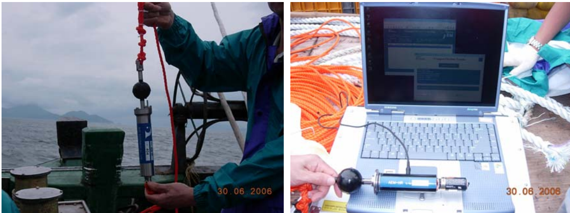
Fig. 2.1.3. (a) Acoustic doppler current profiler(ADCP) and (b) Electromagnetic Current Recorder used in the experiment.
