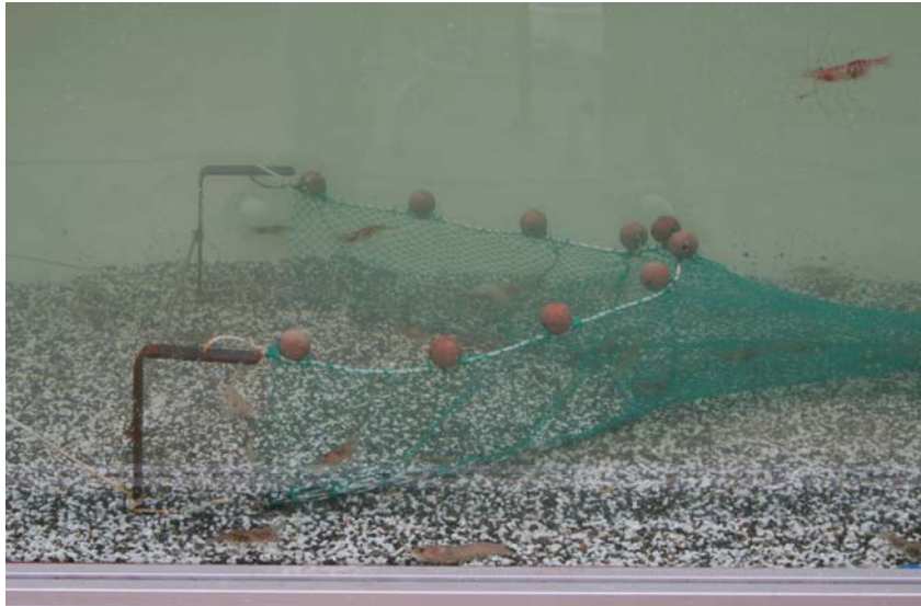
Photo 3. A model net is towing in the tank
