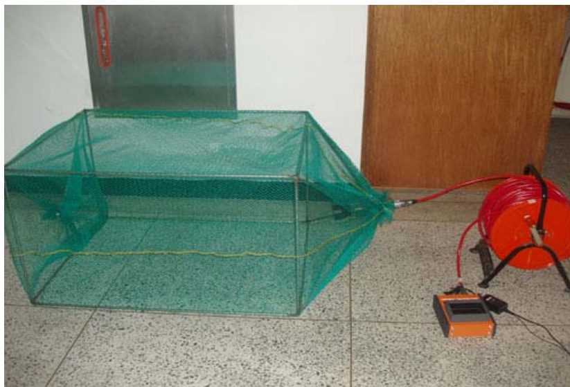
Photo 4. A model net of cod end used shrimp behavior experiment.
