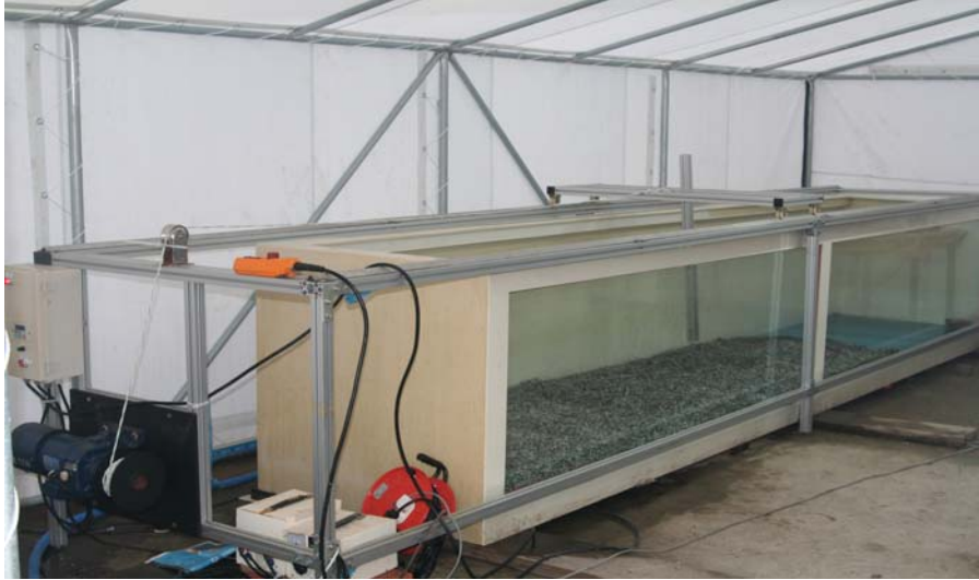
Photo 1. A towing water tank used shrimp behavior experiment.
