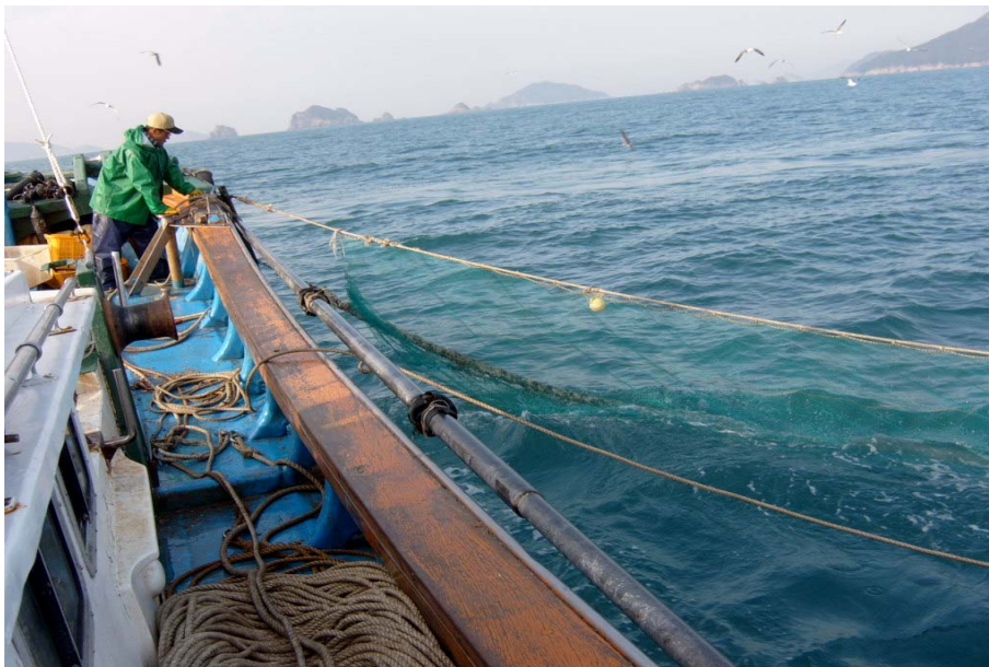
Photo 5. Casting the shrimp beam trawl net in catcher boat
