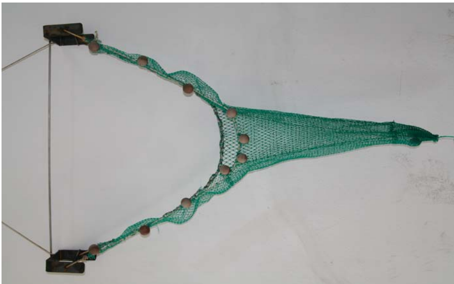
Photo 2. A model net used shrimp behavior experiment.
