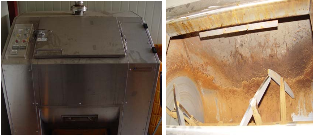
Fig. 1. Biofeeder BF-30 model as a high speed fermenter to prepare fish meal from by-products in fish farms. The left is the outside and the right is the inside of the fermenter (left; outside. light; inside).
