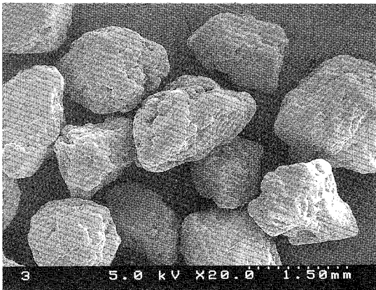
Fig 2. Scanning electron micrographs of encapsulated limestone granule CAP : \times 20 and \times 500 , 2 : EC ( \times 20 and \times 500 ), 3 : Shellac ( \times 20 and \times 500 )
