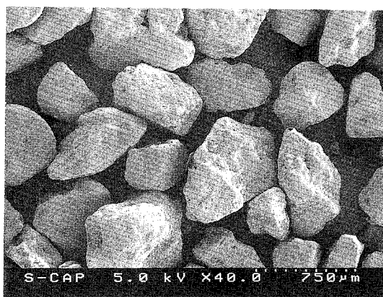
Fig. 7. Scanning electron micrographs of sorbitol
