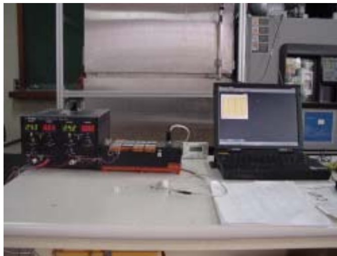
Fig. 3-3 View of data accumulation apparatus for temperature, relative humidity and weighting.
