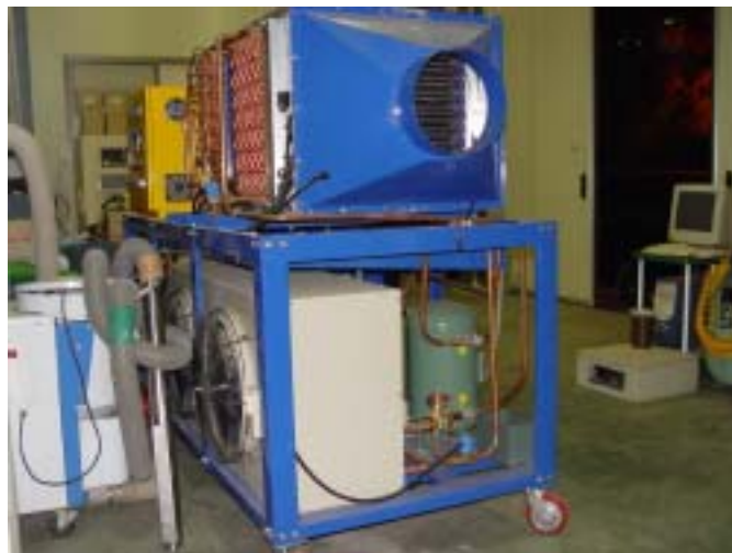
Fig. 3-58 View of heat pump(side).
