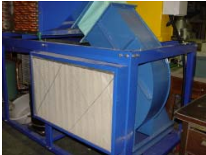
Fig. 3-60 View of fan and filter.
