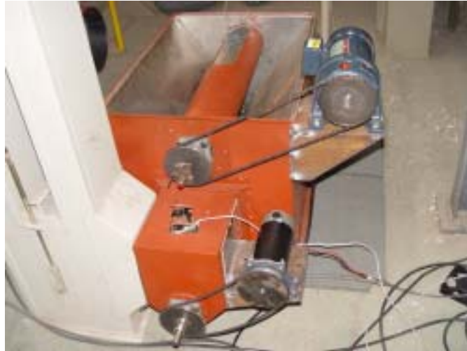
Fig. 3-18 View of the drying exhaust and feeder section.
