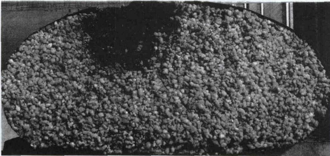
Fig. 10. The cross section of stained substrate in perlite bag.
