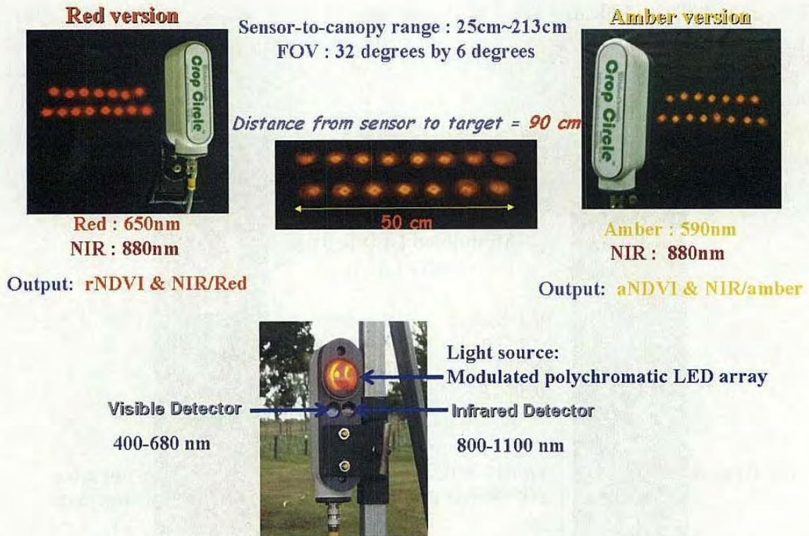
Fig 2-3. Picture of Crop Circle amber version (left) and red version (right) sensors and their illumination and field of view (FOV).
