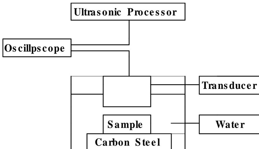
**Fig.1. Block diagram of experimental system for ultrasonic wave measurement.**
