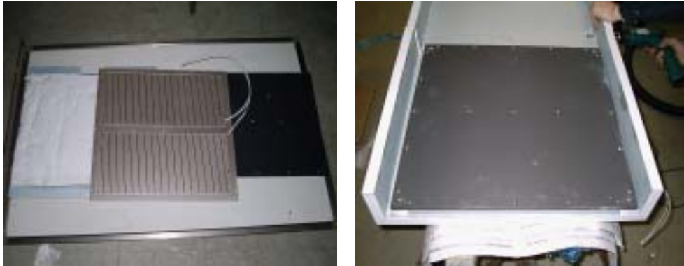
Photo. 31. Assembling of far infrared heater and heating chamber.
