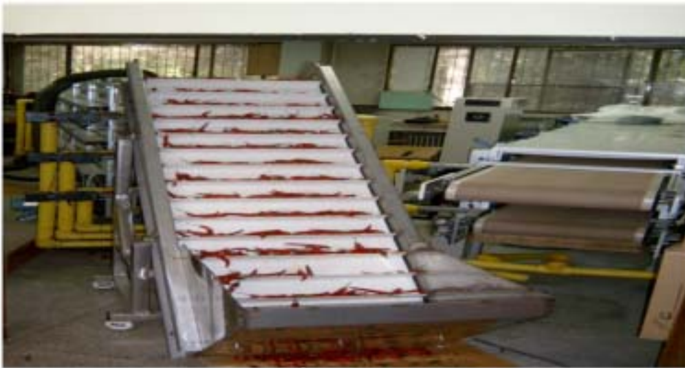
Photo. 69. Five stage-far infrared dryer of up draft airflow type.
