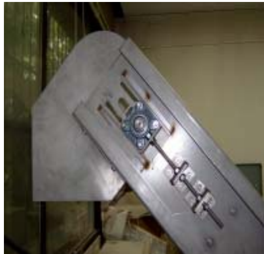
Photo. 55. Input guide & Belt tension controller.
