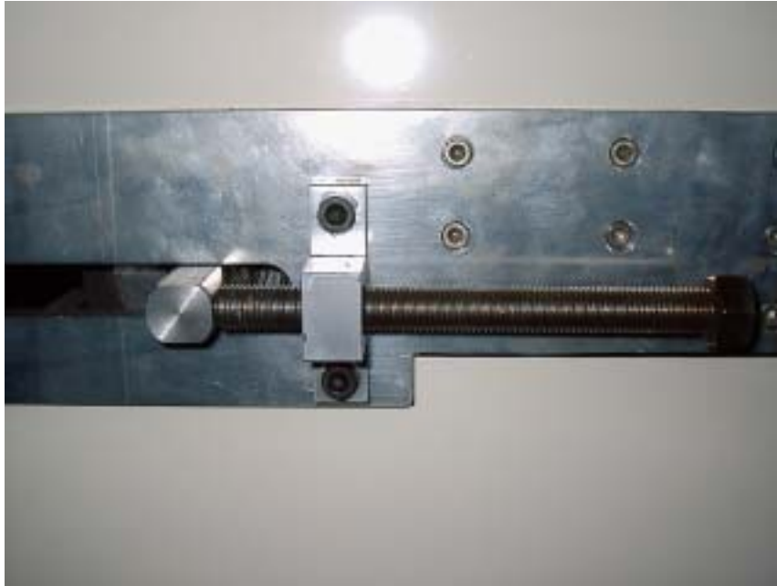
Photo. 36. Belt tension controller.
