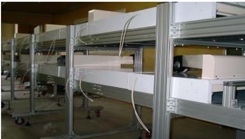
Photo. 30. Assembling of two stage-far infrared dryer of down draft airflow type.
