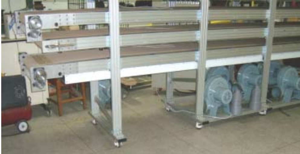
Photo. 40. Assembling of three stage-far infrared dryer of down draft airflow type.
