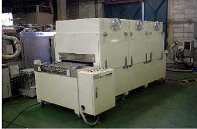
Photo. 70. The Hybrid heating system.
