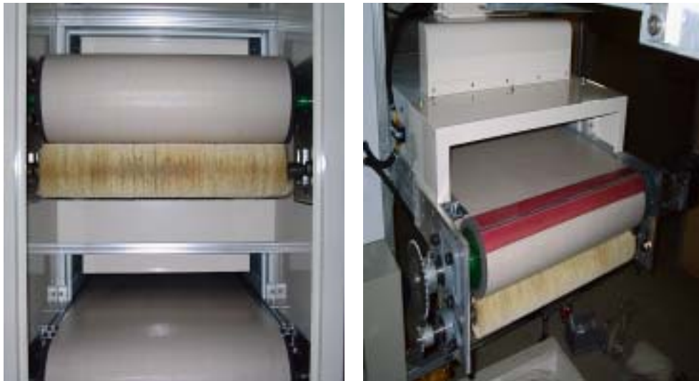
Photo. 35. Belt conveyor and belt brush.
