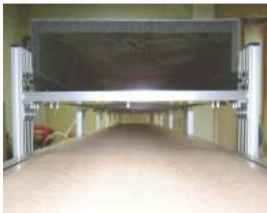
Photo. 48. The upper preheating duct.
