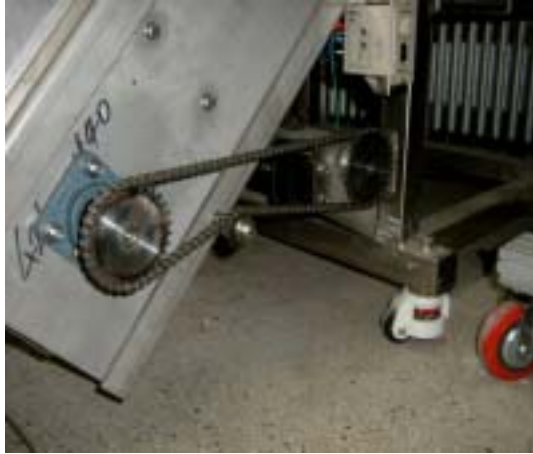
Photo. 52. Chain tension controller.
