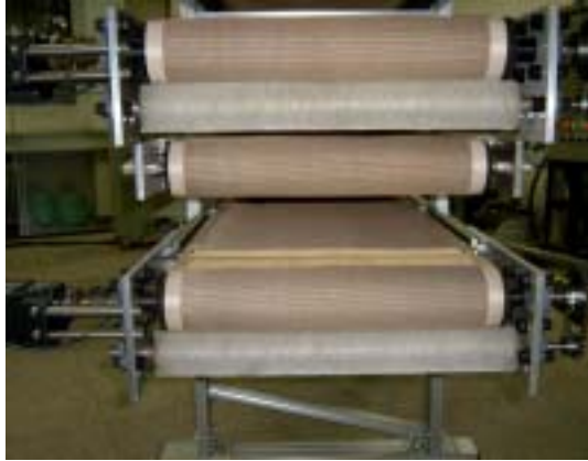
Photo. 43. Driving shaft and brush.
