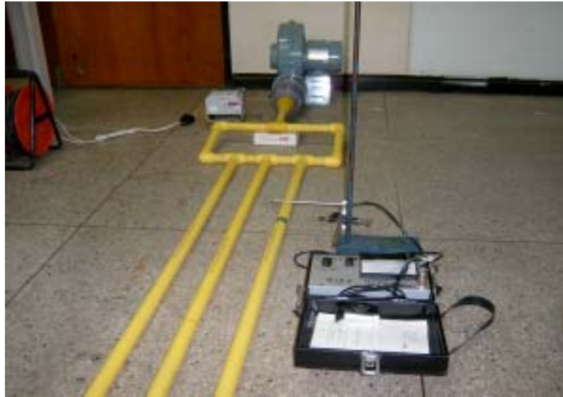
Photo. 60. Measurement of blast velocity of blast pipe by an anemometer.
