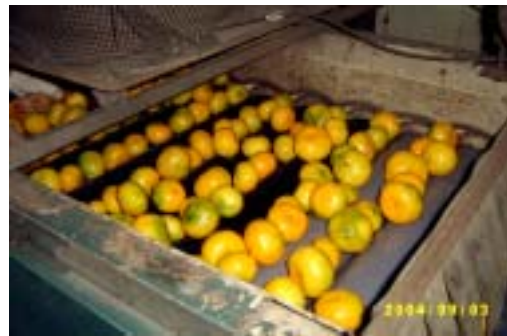
<Dewatering and air-blowing>
