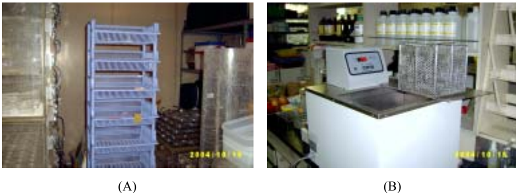
Fig. 1. Appearance of heat treating systems used for citrus fruits in this study. (A): hot air treatment in a heating room, (B): hot water treatment in a water bath.
