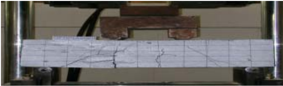
Fig. 11-8 Photo of flexure and shear cracks from GFRP Aslan rebar reinforced concrete specimens
