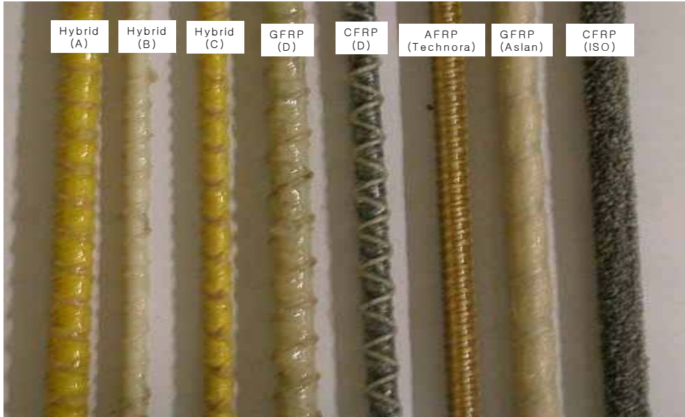
Fig. 6-1 Surface characteristics of FRP rebars
