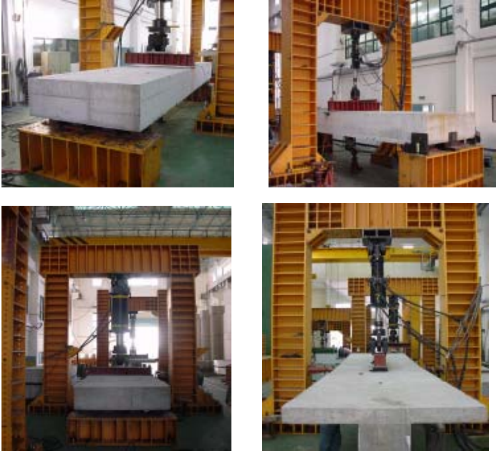
Fig. 13-1 Flexural test set-up of FRP rebar reinforced concrete beam
