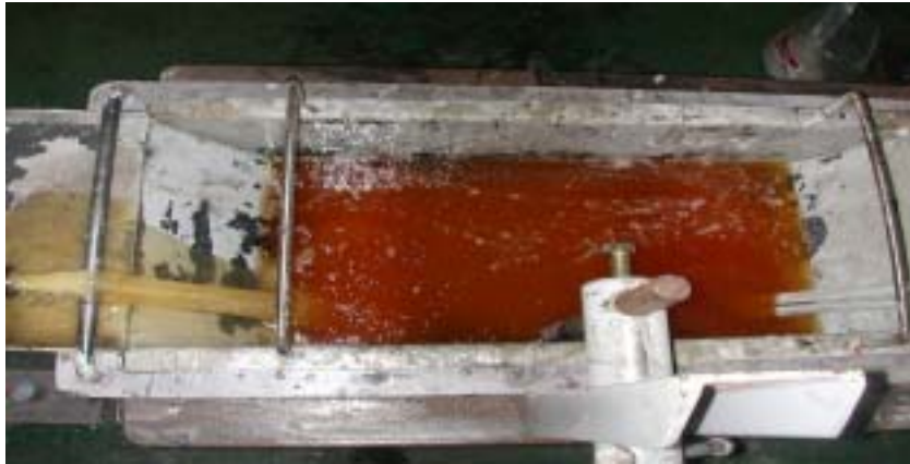
Fig. 3-7 Reinforcement fiber impregnation system
