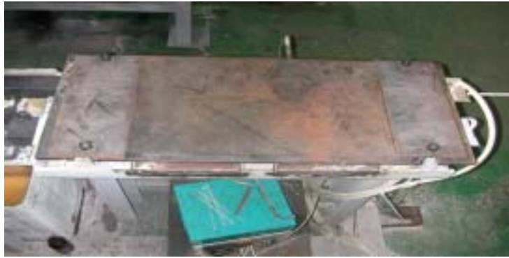
Fig. 3-8 Heated die system
