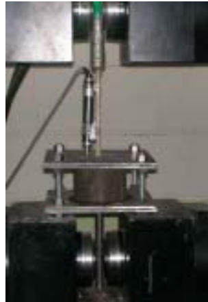
Fig. 9-4 Pullout test set-up of FRP rebar
