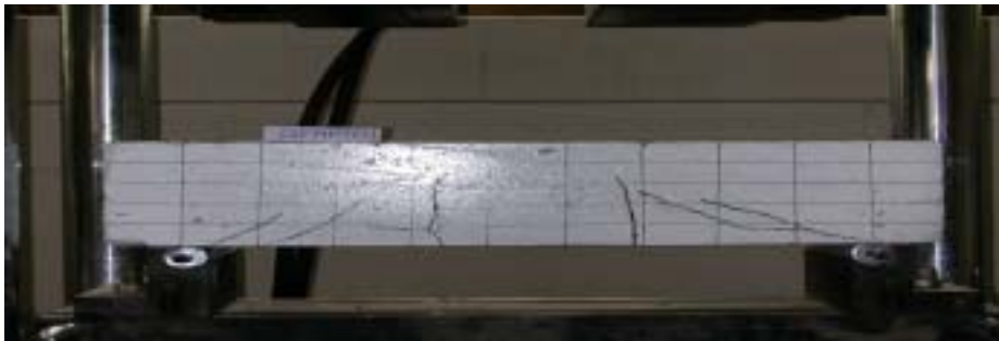
Fig. 11-11 Photo of flexure and shear cracks from GFRP(D) rebar reinforced concrete specimens
