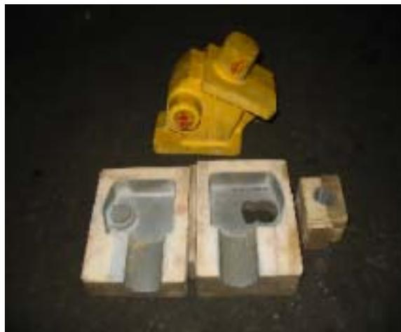
Fig. 5-10 Mold photo of Steering system mechanism
