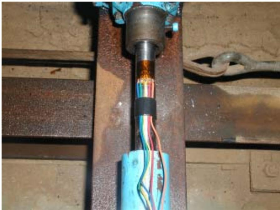
Fig. 3-5 View of strain gage attached on handle axle.
