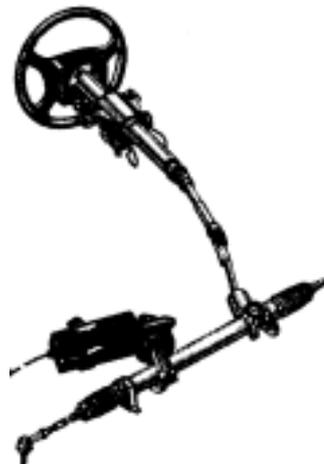
(c) Rack assist-pinion driving type      (d) Rack assist-ball screw type
