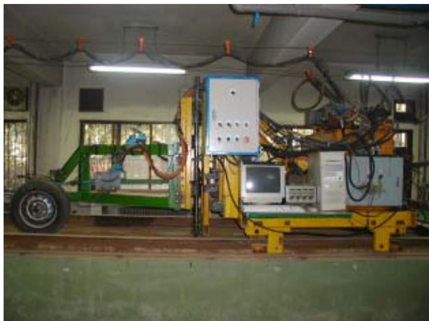
Fig. 3-12 Overall view of single-tire steering test device.
