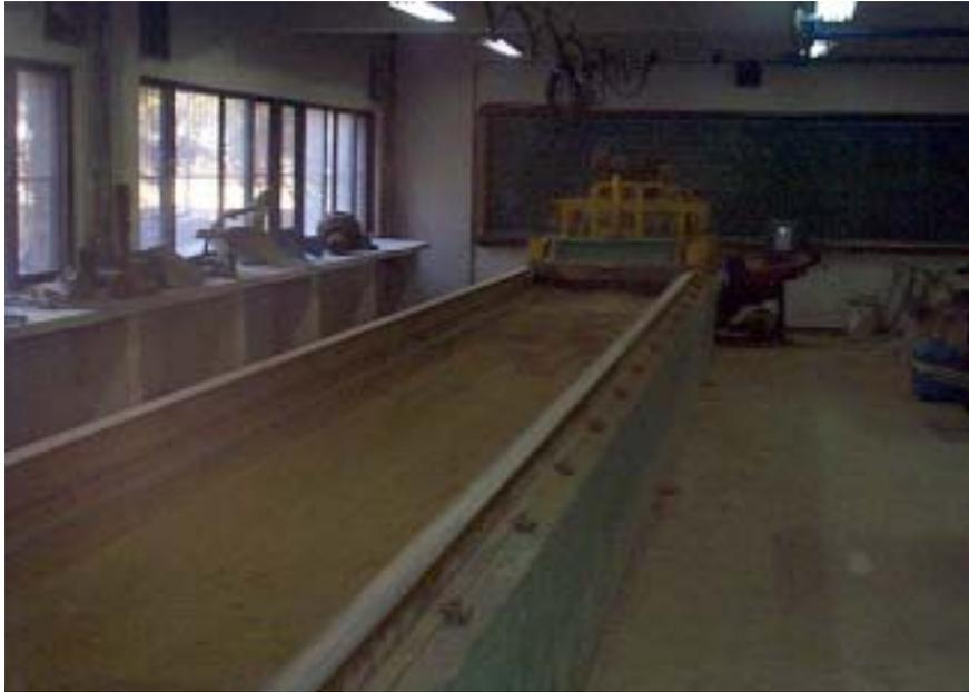
Fig. 3-1 View of soil bin and rail system.
