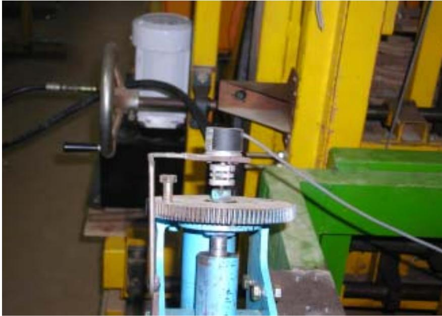
Fig. 3-9 Device for measuring the steering angle of handle.
