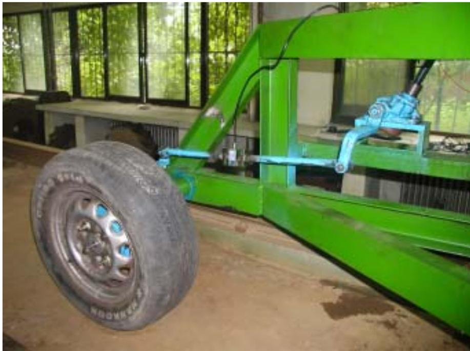
Fig. 3-8 View of loadcell for measuring the push-bar force.
