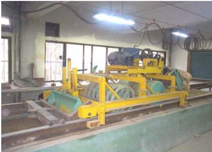
Fig. 3-2 View of soil processing carriage.
