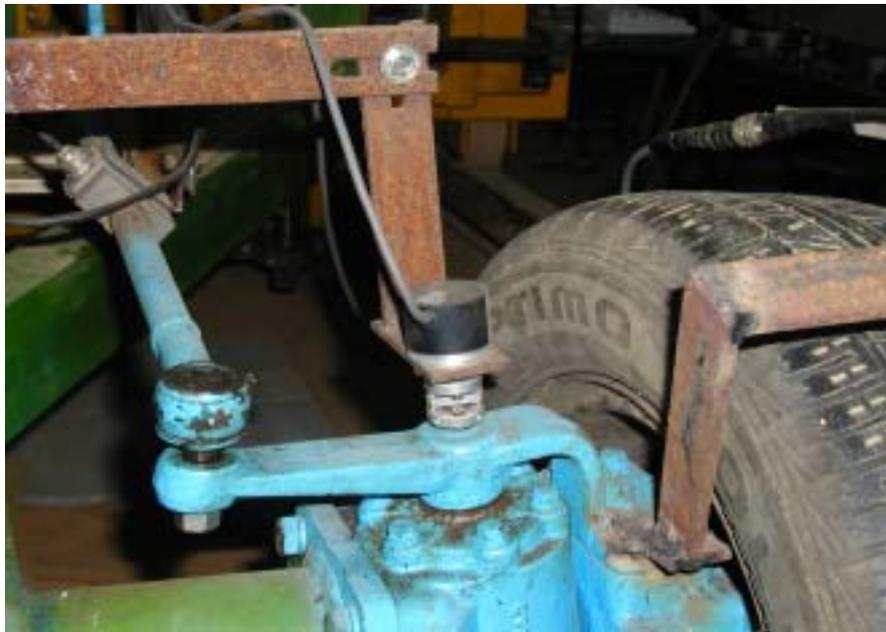
Fig. 3-10 Device for measuring the rotating angle of king\_pin axle
