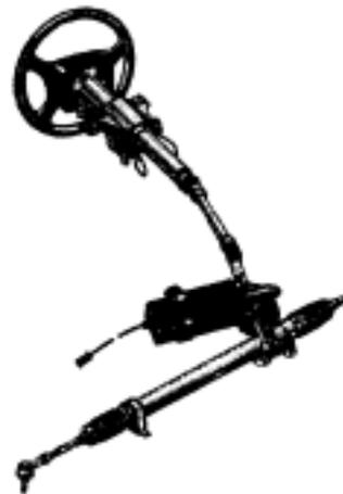
(a) Pinion assist-column driving type      (b) Pinion assist-pinion driving type
