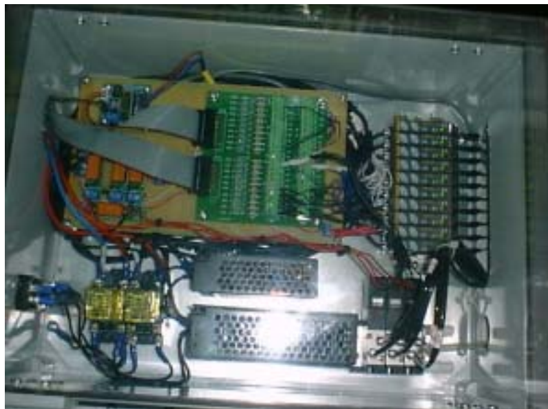
Fig. 14 Control box for data communication between control computer and gripper.
