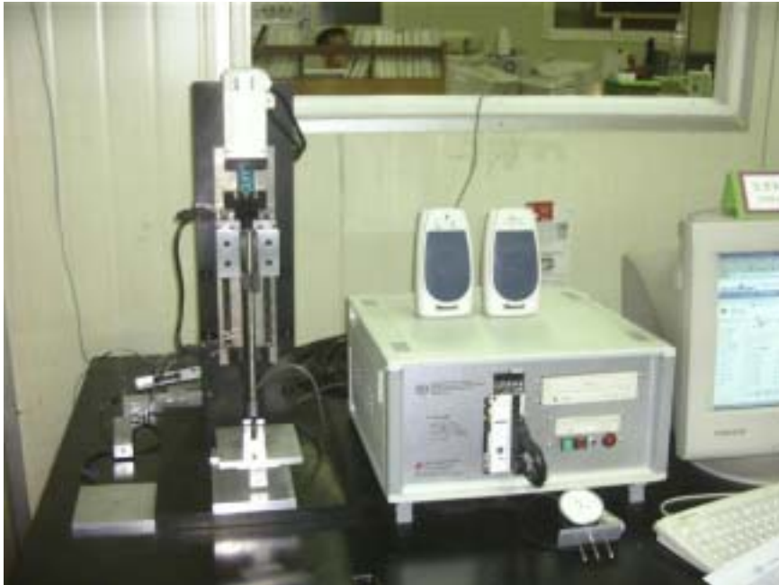
Fig. 1 The picture of shear-force measurement jig installed to UTM.
