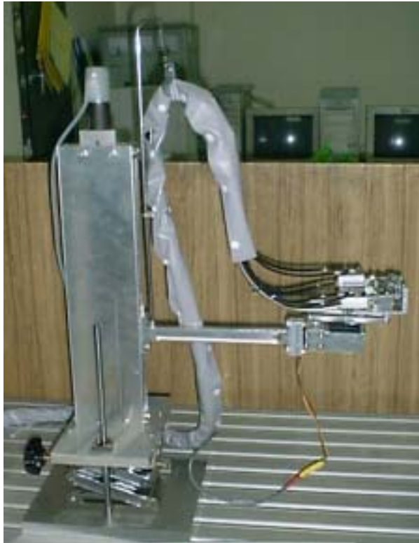
Fig. 18 Gripper manufactured for performance test.
