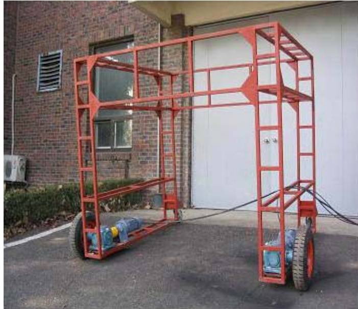
Fig. 21 Photograph of frame and traveling mechanism.
