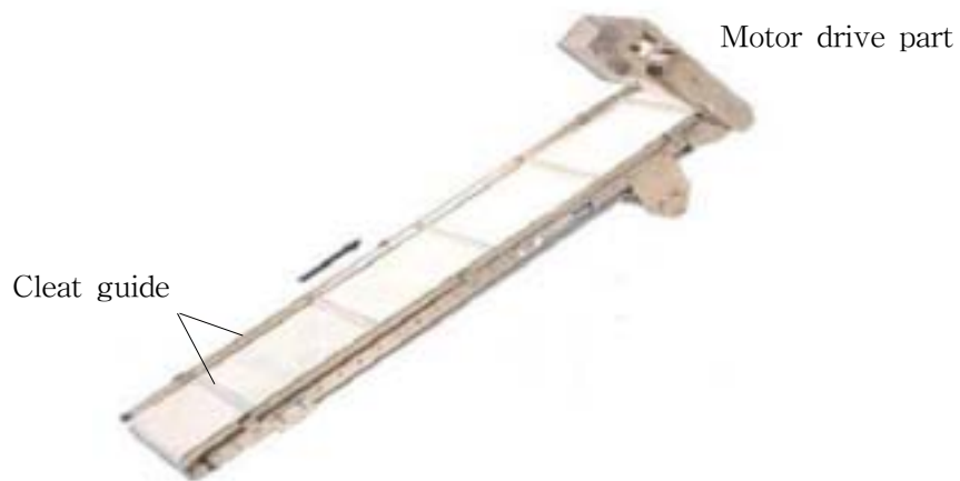
Fig. 23 Photograph of conveying equipment designed.
