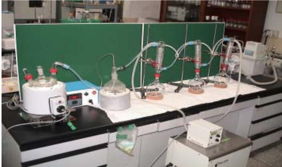
Figure 1-5. The designed extractor for the Bioessential oil extraction.
