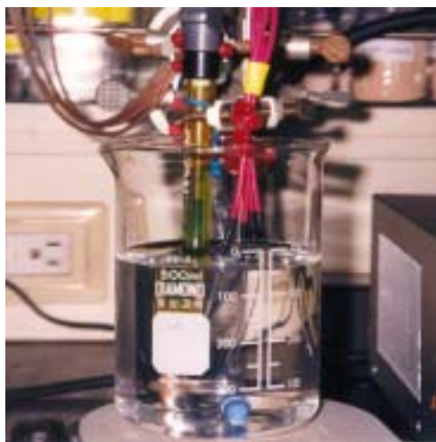
Fig. 93. Photograph of the solid-state taste sensor array.
