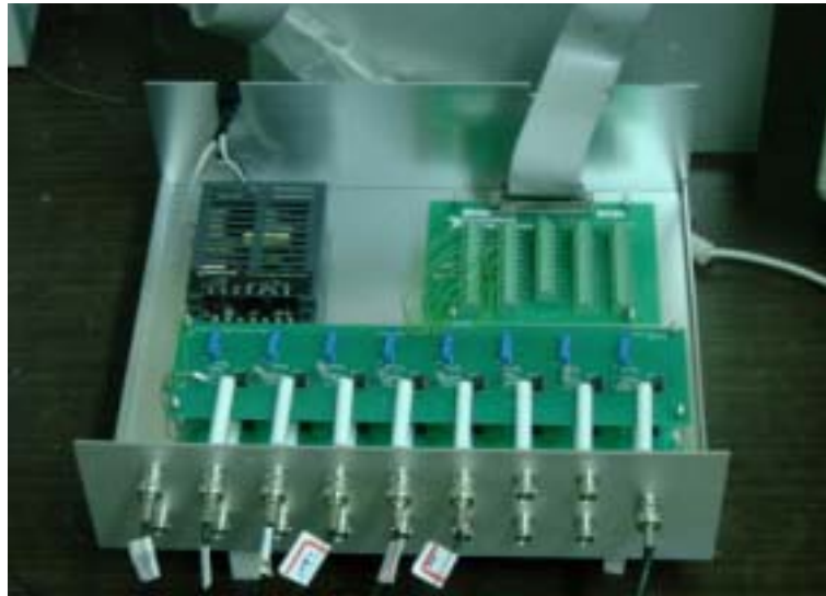
Fig. 29. Inner view of 16 channel amplifier with high input impedance.
