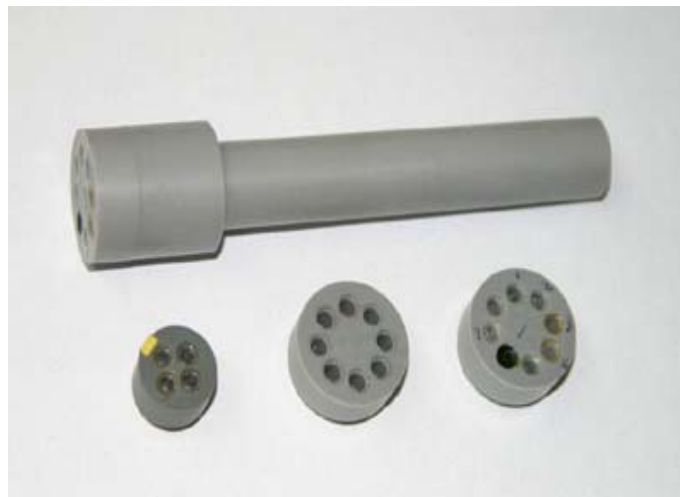
Fig. 91. Photograph of the 8 channel taste sensor in-situ micro-array having various polymer membranes.
