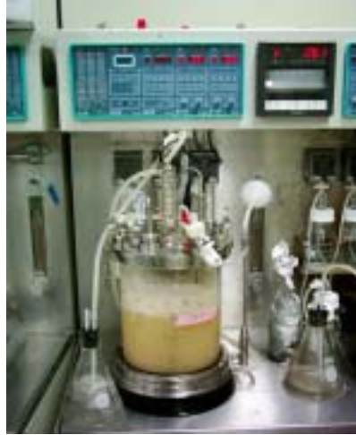
Figure 4. The submerged liquid culture in the 5 ℓ J-fermenter.
