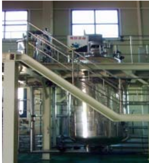
Figure 7. The submerged liquid culture in the 5 kL fermenter.
