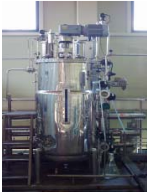
Figure 6. The submerged liquid culture in the 500 ℓ fermenter.
