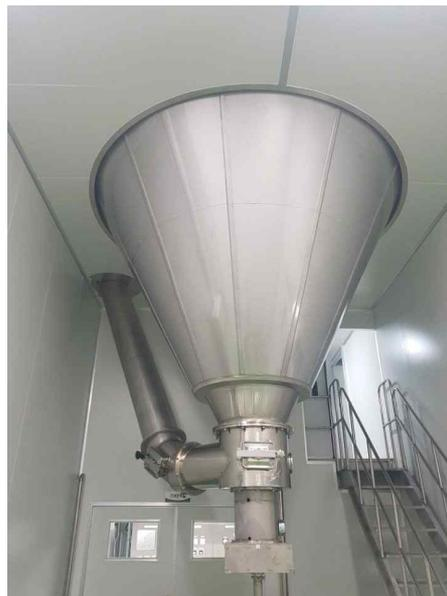
Fig. 7. Picture of spray dryer system
