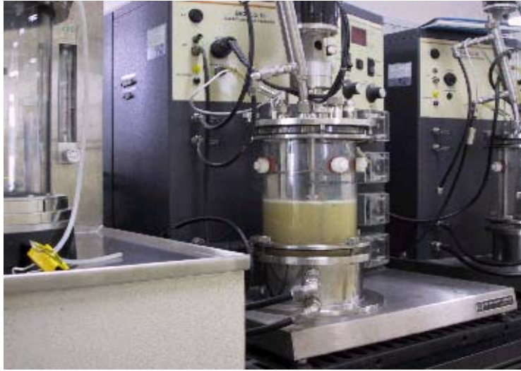
Figure 28. Bioflo III artificial rumen fermenter
