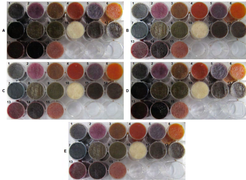
Fig. 223. Change of coloring of lip stick having the natural plant pigment and extract of Dioscorea japonica as affected by UV A light time
