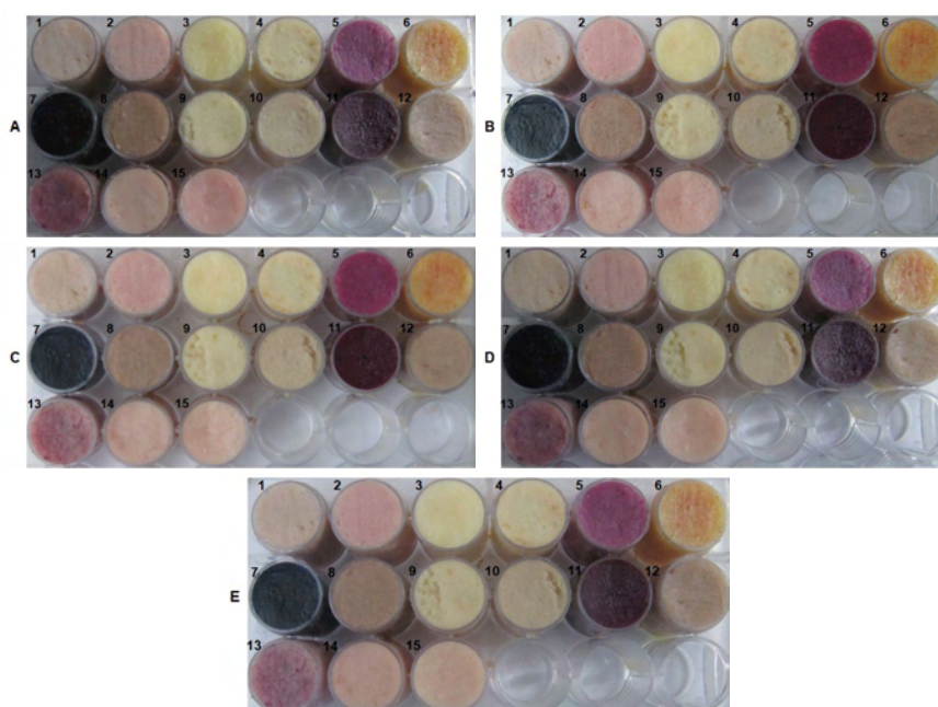
Fig. 221. Change of coloring of lip balm having the natural plant pigment and extract of Dioscorea japonica as affected by UV A light time
