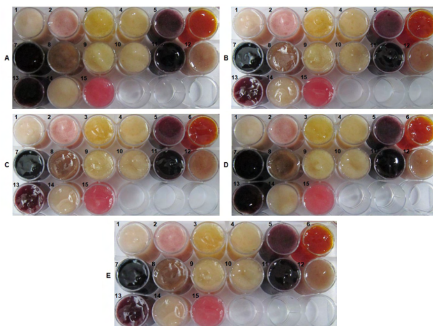
Fig. 222. Change of coloring of lip gloss having the natural plant pigment and extract of Dioscorea japonica as affected by UV A light time
