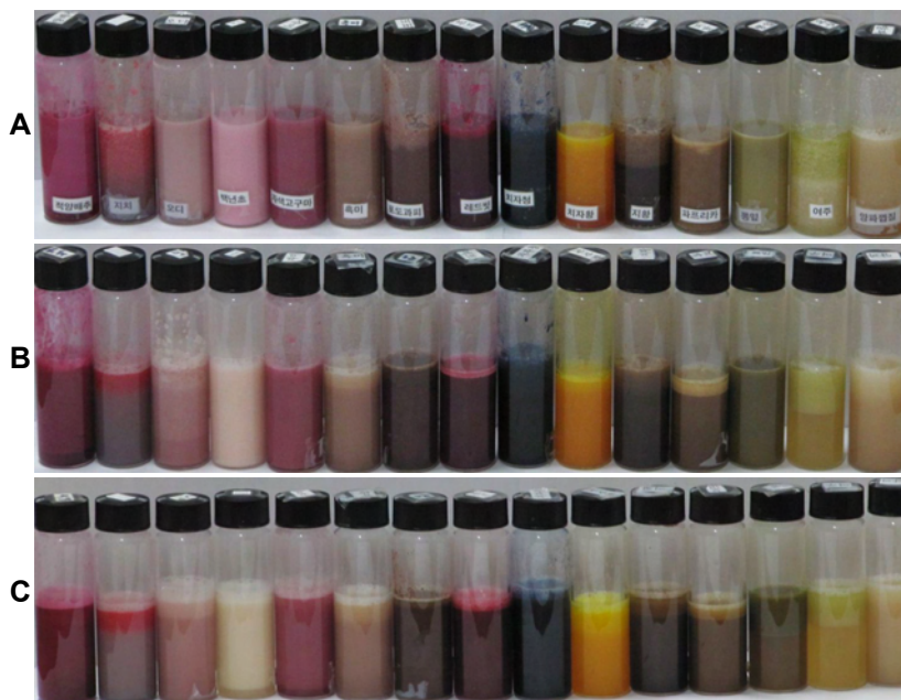
Fig. 164. Change of coloring of the cosmetic composition as affected by heating time
