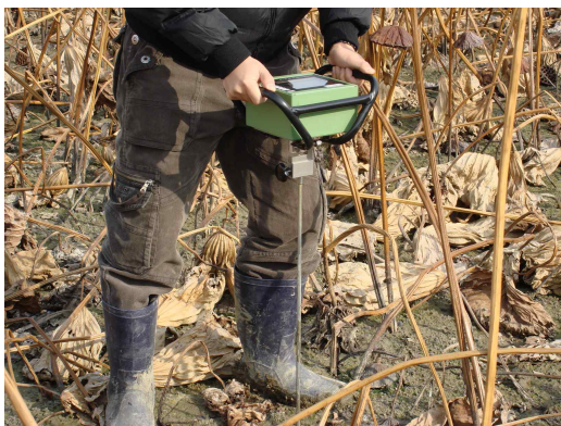
Fig. 5-6. Hardness measurement of soil for rice paddy field with soil hardness tester.
