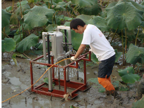
Fig. 5-27. Picture for the lotus field experiment of lotus root harvester with an ejection apparatus of high pressure air.
