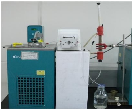
Fig. 25. (a) A packed-bed reactor with CSabn and CSabf immobilized on Duolite A568 (b) Effect of dilution rate on L-arabinose production in a packed bed reactor.
