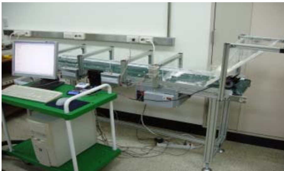
Fig. 19. Photo of conveying system and microwave measurement system
