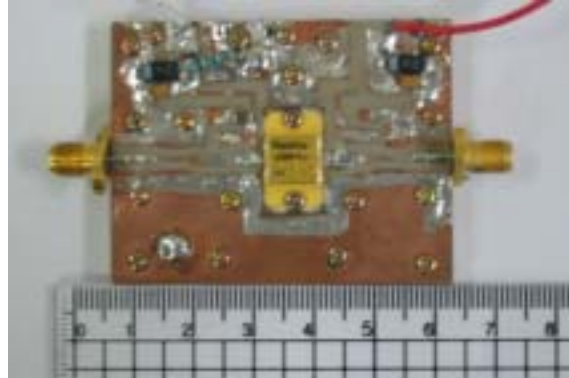
Fig. 50. Photo of fabricated power amplifier
