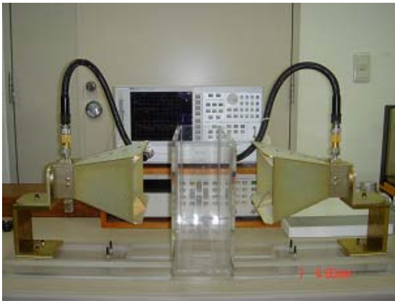
Fig. 7. Microwave measurement setup.
