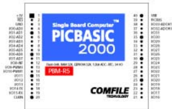
Fig. 13. Layout of the PICBASIC module
