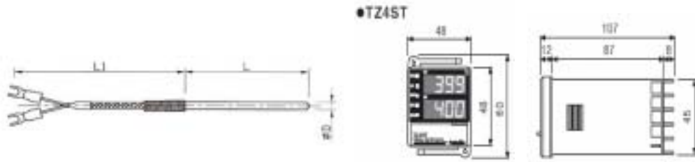
(a) K-type thermo-couple (b) Temperature sensing module
