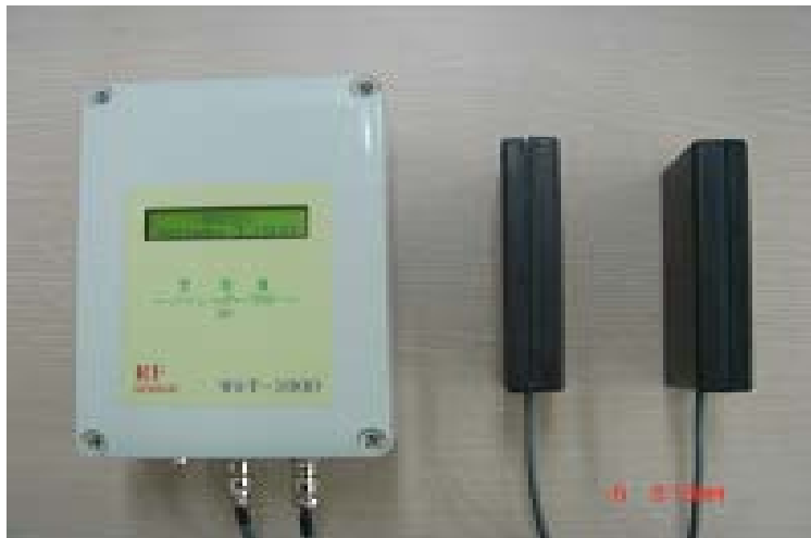
Fig. 8. Photo of prototype moisture meter with patch antenna
