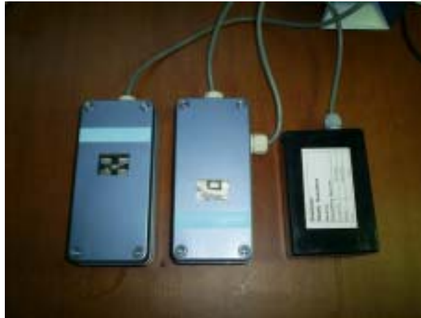
Fig. 12. Photo of the wireless prototype moisture meter
