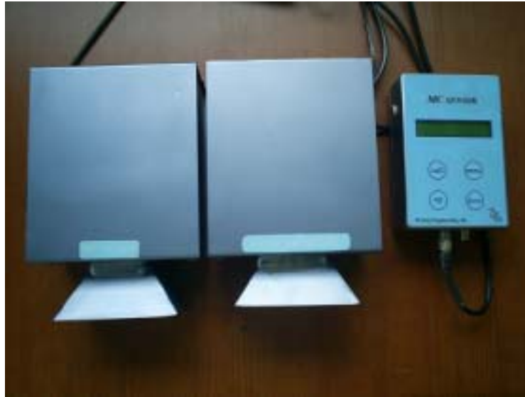
Fig. 9. Photo of prototype moisture meter with horn antenna
