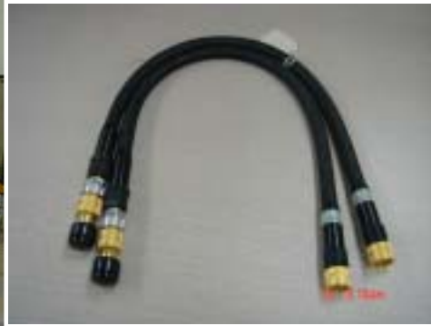
Fig. 8. 7mm flexible test port cable.
