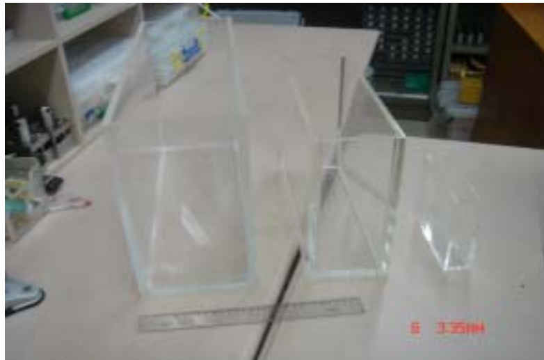
Fig. 6. Three kinds of sample holder for powdered food
