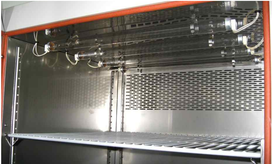
Fig. 39 Image of UV lamp installed in thermo-hygrostat.
