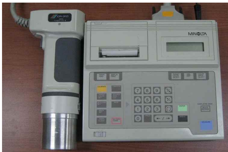
Fig. 19 Chromameter used for meat color measurement.
