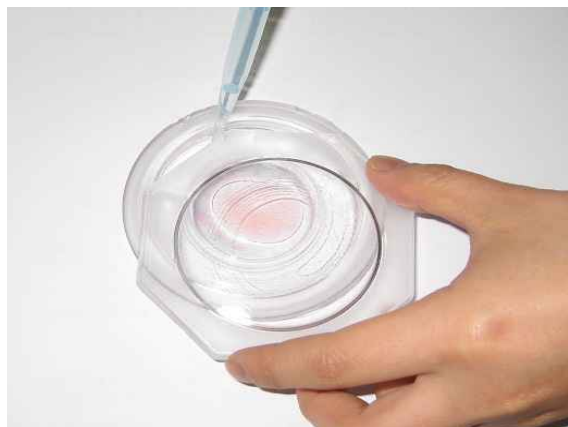
Fig. 16 Image of conway dish with titration.
