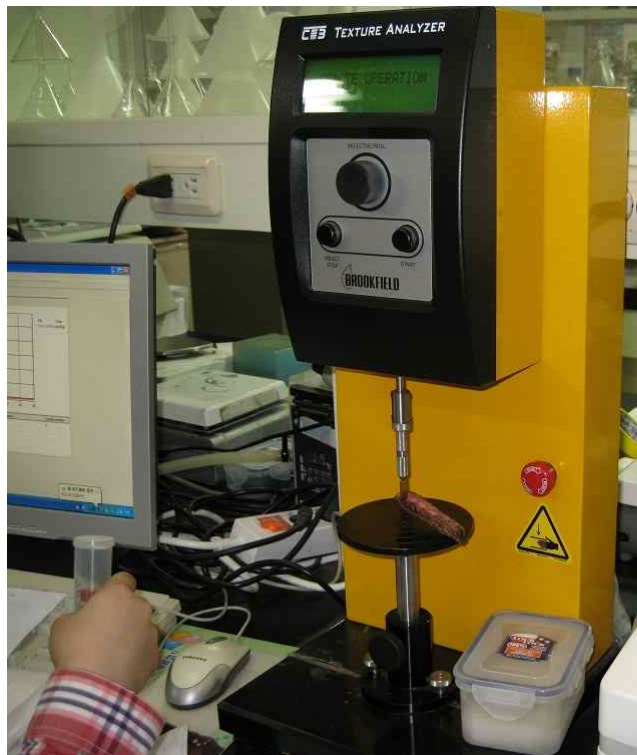
Fig. 22 Image of measuring shear value of sample using Texture Analyzer.
