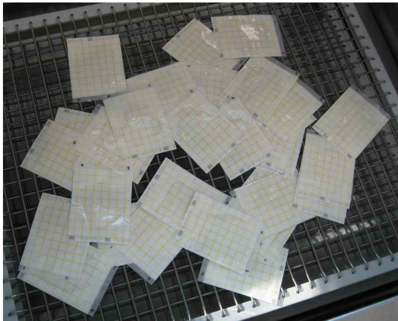
Fig. 18 Image of petrifilm in incubator for total microbial count.
