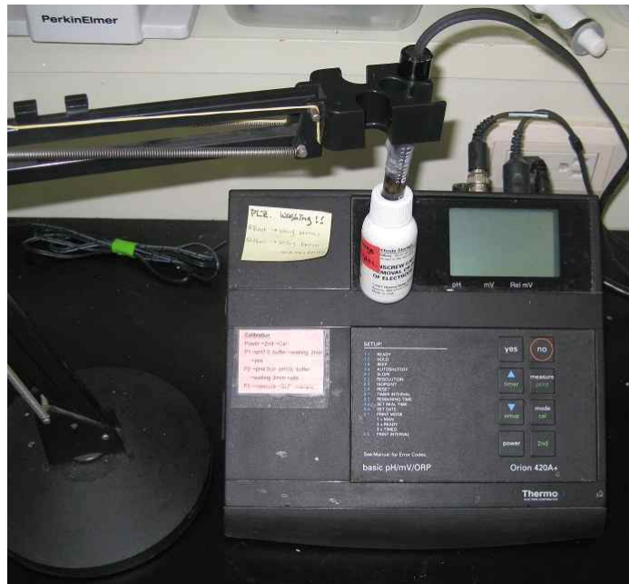
Fig. 15 Image of pH Meter for measuring sample pH.
