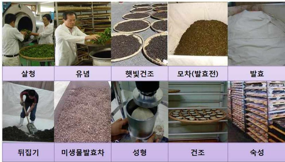
Fig. 2-3. Manufacturing process of microbial fermented tea.
