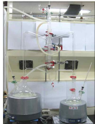
Fig. 1-4. Simultaneous distillation and extraction (SDE) apparatus.
