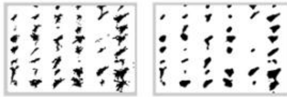
An illustration of morphological closing. (a) Original filtered binary image, (b) After morphological closing operation.
