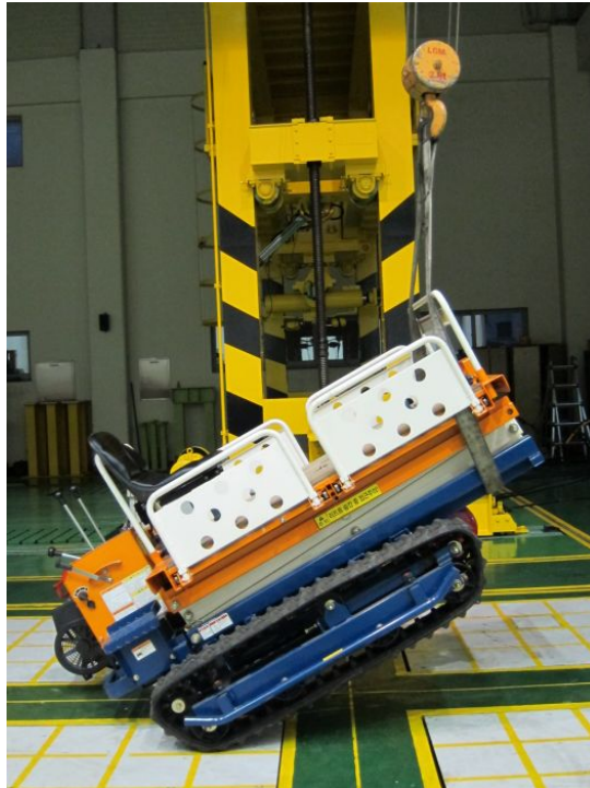
Fig. 138 Determination of mass center of Aerial-lift in y-axis direction
