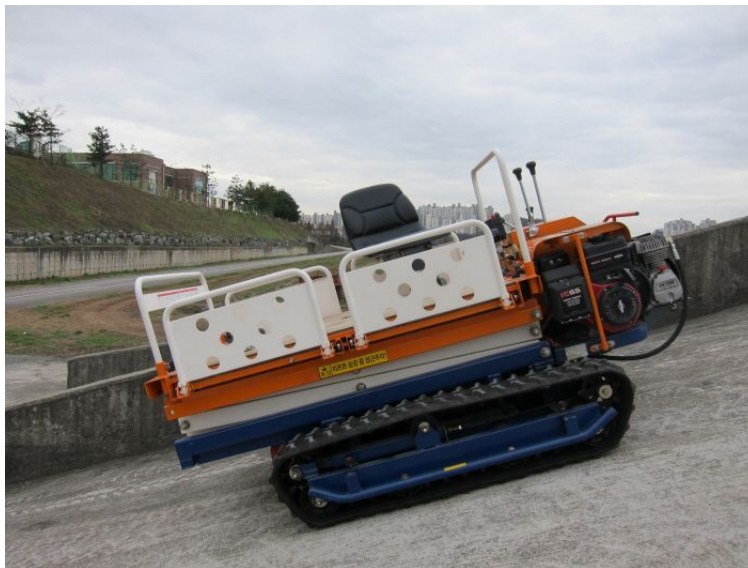
Fig. 154 Descending test at 21% slope.
