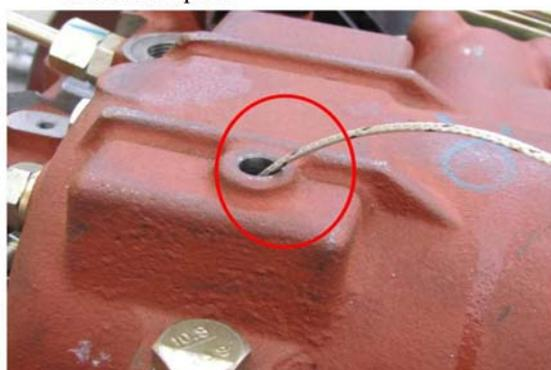
(d) Temperature sensor for measuring hydraulic temperature
