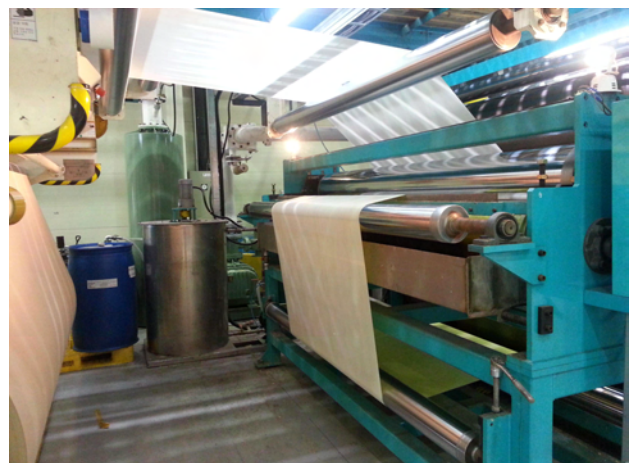
Fig. 3.171. Linerboard, corrugating medium (left) and joining non-woven fabric with corrugating medium (right).
