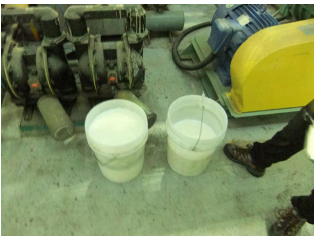
Fig. 3.236. Starch-latex mixture (left) and its injection to corrugator (right).
