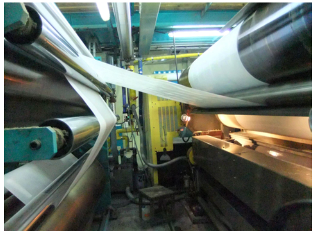
Fig. 3.238. Coating process of non-woven fabric with water.
