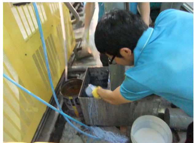
Fig. 3.236. Starch-latex mixture (left) and its injection to corrugator (right).
