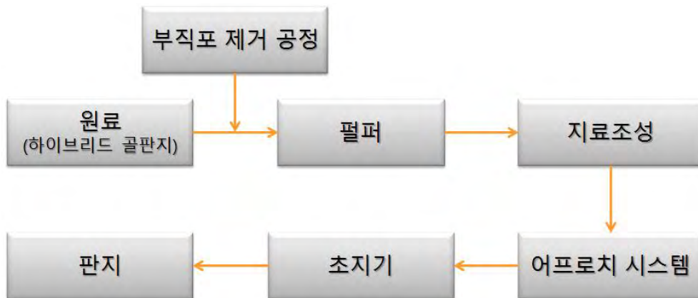
Fig. 3.250. Flow diagram of recycling system of hybrid corrugated board.
