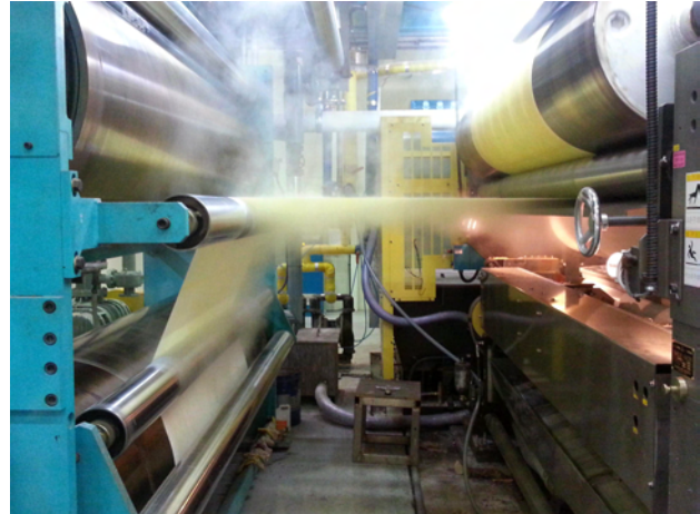
Fig. 3.169. Non-woven fabric (left) and its coating process with sulfur solution (right).
