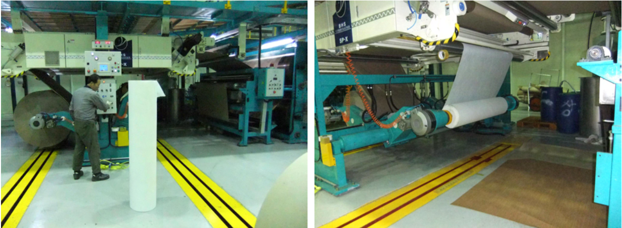
Fig. 3.141. Pictures of the input of non-woven fabric to corrugator.
