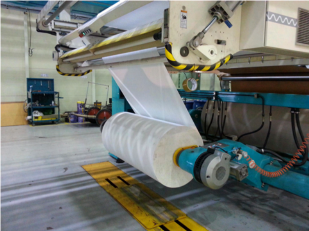
Fig. 3.169. Non-woven fabric (left) and its coating process with sulfur solution (right).
