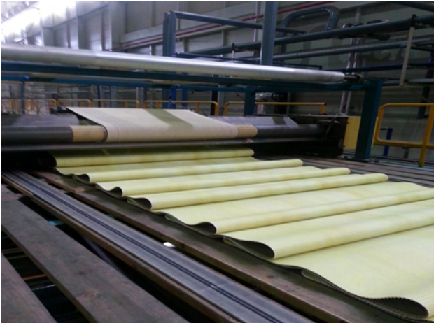
Fig. 3.172. Single faced corrugated board with non-woven fabric and corrugating medium.
