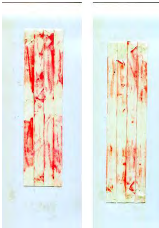
Fig. 3.224. Film images of 100 cm drop test – conventional corrugated board (left) and hybrid corrugated board (right).
