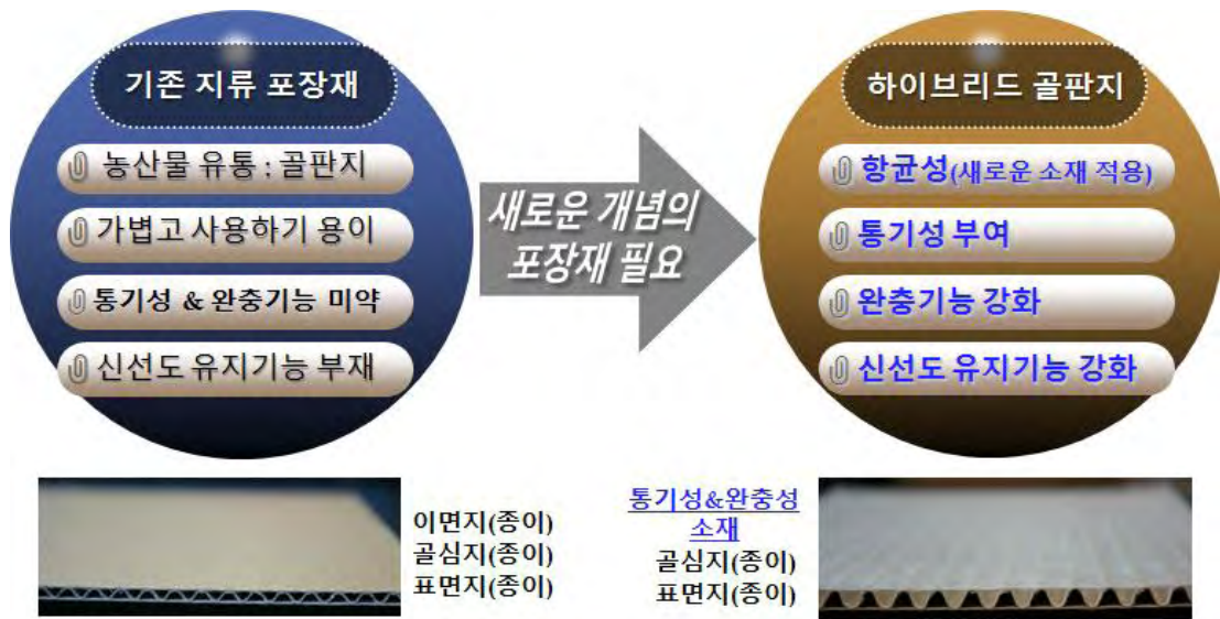
Fig. 1.1. Conventional corrugated board (left) and functional hybrid corrugated board (right).
