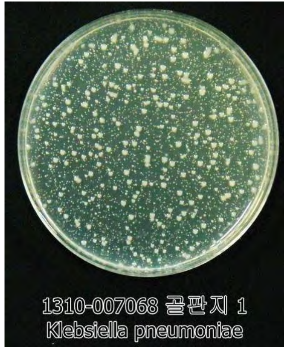
Fig. 3.181. Photographs of sample C1 after 18 hours - Staphylococcus aureus (left) and Klebsiella pneumoniae (right).
