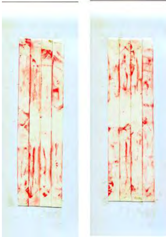
Fig. 3.223. Film images of 60 cm drop test – conventional corrugated board (left) and hybrid corrugated board (right).
