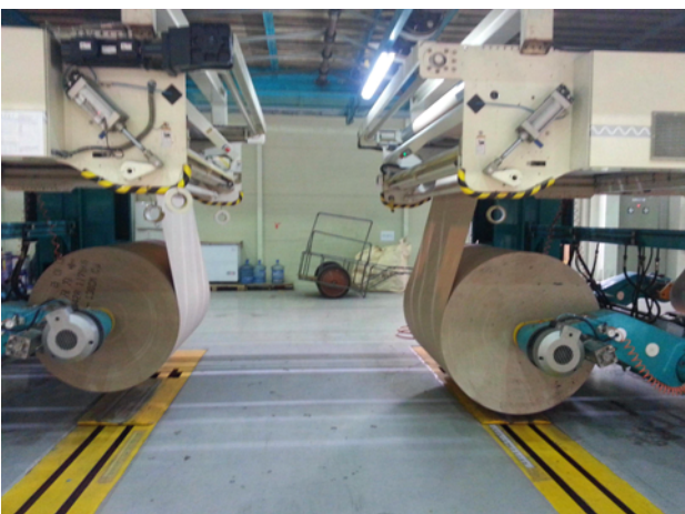
Fig. 3.171. Linerboard, corrugating medium (left) and joining non-woven fabric with corrugating medium (right).
