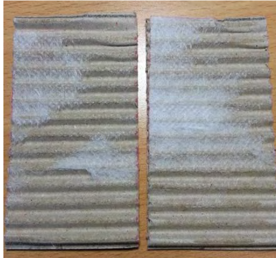
Fig. 3.233. Photographs showing the adherend between corrugated board and non-woven fabric coated with starch and 10% latex mixture (left) and starch and 20% latex mixture (right).
