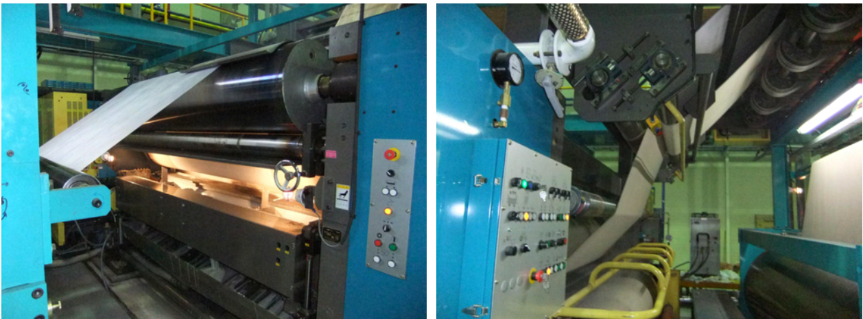
Fig. 3.142. Tension adjustment of non-woven fabric (left) and corrugating medium (right).
