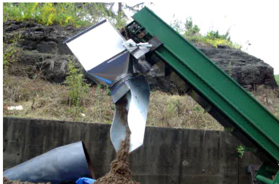
Fig. 47 The final loading system with rotatable suit type on improved prototype
