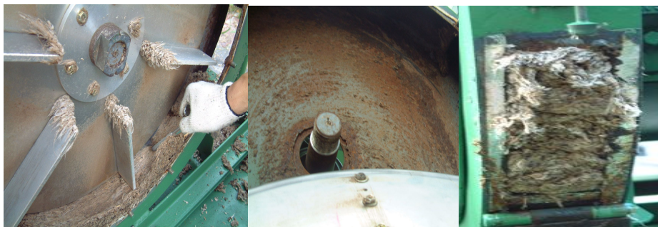
(A) Material hardening (B) Bolts abrasion (C) Material accumulation
