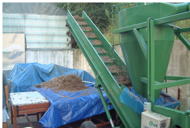
Fig. 52 Loading test on the workplace with improved prototype
