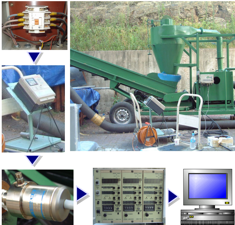
Fig. 17 Schematic diagram of pressure measuring process for the fan
