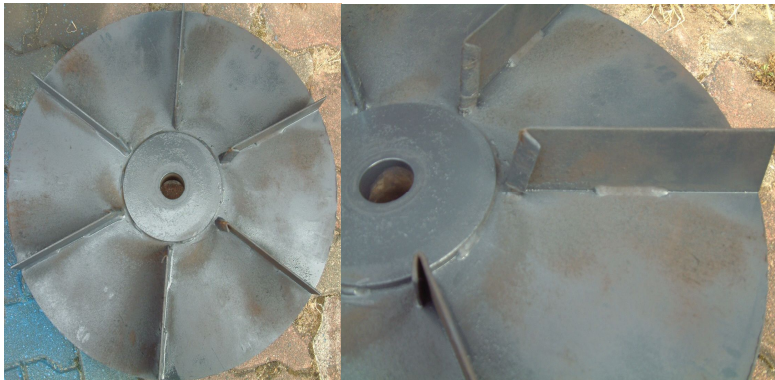
Fig. 35 Schematic shape of the fan for the prototype with 600mm diameter, 6EA wings(60° array)
