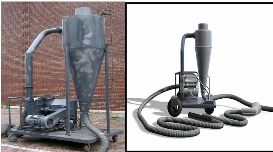
Fig. 29 Schematic picture and 3D animation of the sub-rate materials loading & unloading device on prototype
