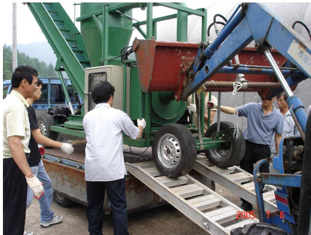
Fig. 72 Loading of developed machine by the loader attached tractor
