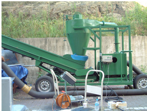
Fig. 59 Capability test for the loading machine of the improved prototype
