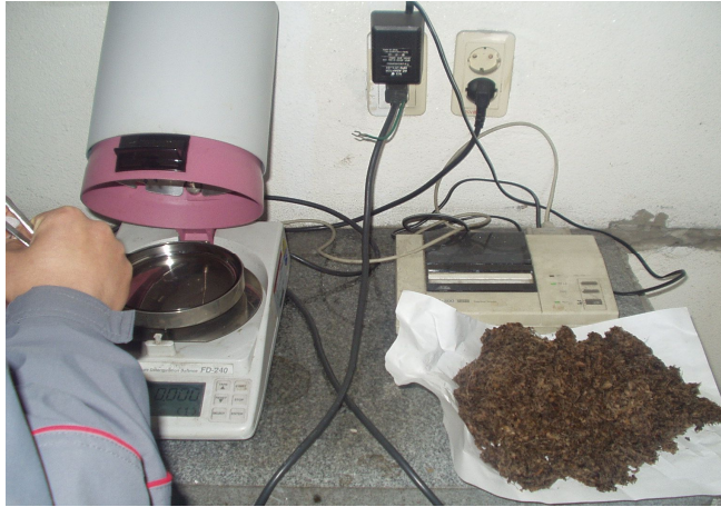
Fig. 11 Analyzing of moisture content by infrared light equipment
