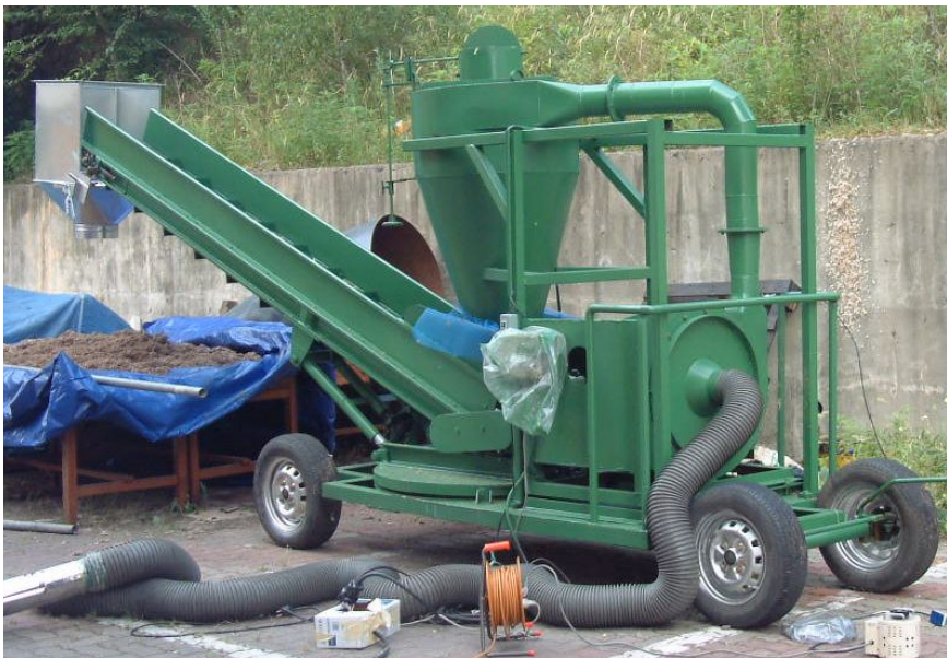
Fig. 32 Schematic picture of the sub-rate materials loading & unloading device on improved prototype
