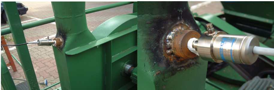
Fig. 16 Measuring of pressure in the fan as change rpm of shaft
