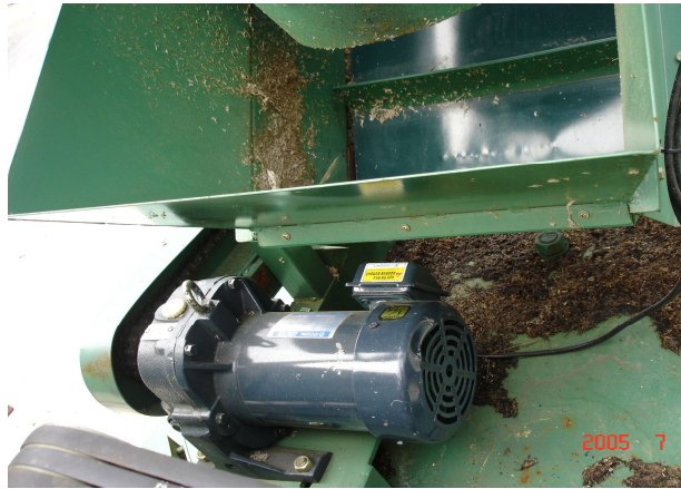
Fig. 50 Motor for control of belt conveyor rpm
