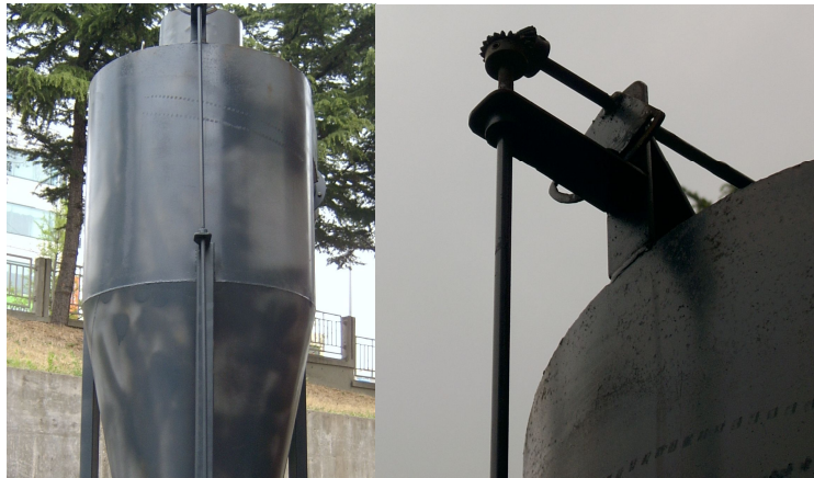
Fig. 42 Picture of a cyclone and a bevel gear set for air flow control
