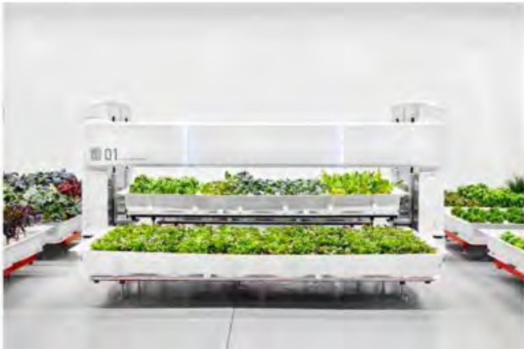
Meet Angus, Iron Ox's robot porter, which is designed to move pallets of plants around their indoor farm. | Photo: Iron Ox.
