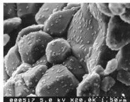
Figure 4: SEM image of Influenza Virus adsorbed by Hydroxyapatite ceramic surface
