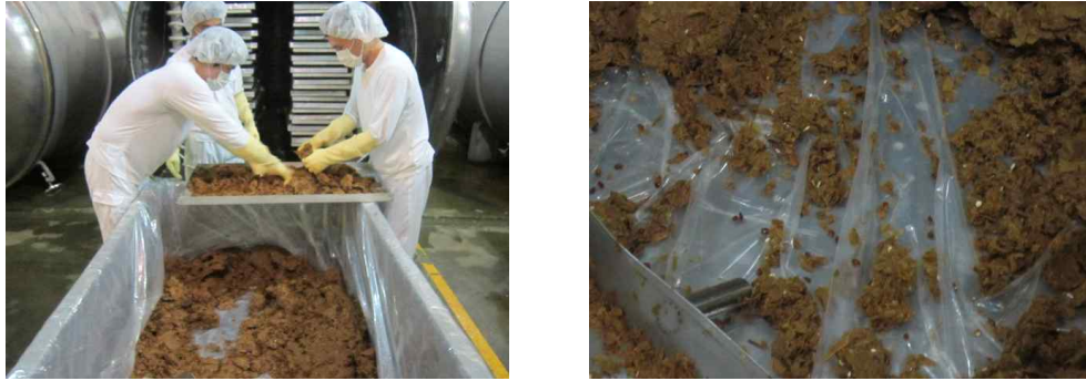
Figure 4-4. Vacuum Drying of pre-treated apple peel
