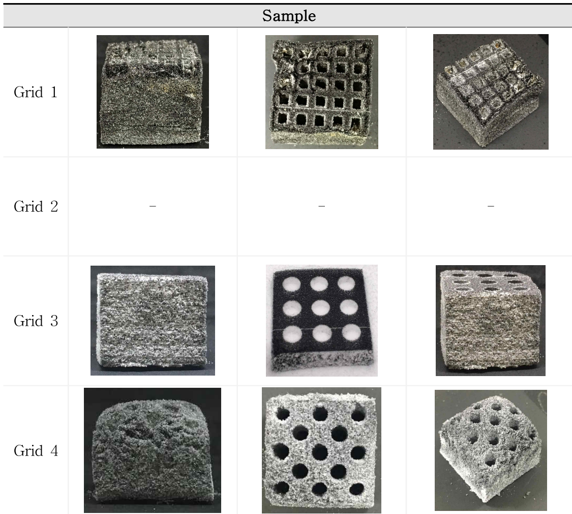
Fig. 13. 3D model of maltodextrin at different design printed by powder-bound microdispensing.
