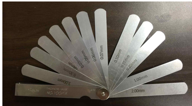
<Swan사의 Thickness gauge NO. 100MX>
