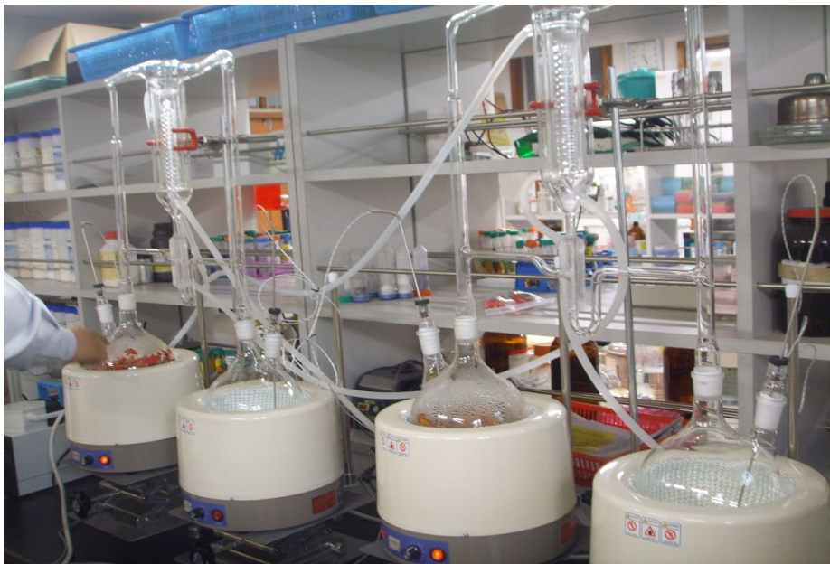
Fig. 1. Hydro distillation apparatus for extraction of essential oil and floral water.
