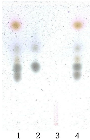
Figure 17. Compositional analysis of the purified colorant: Sugar composition analysis by HPTLC (Lane: 1,4: standard monosaccharides, 2. Acidic hydrolyzate, 3. Purified fraction).
