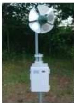
Fig. 1 Proto type of rodents repellent system
