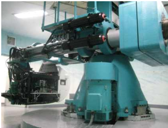
(a) Centrifuge shaking table test equipment
