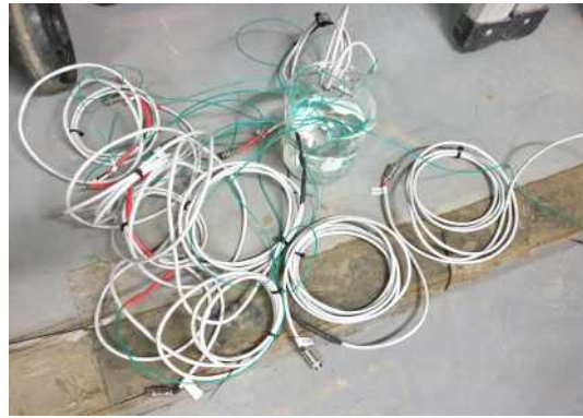
(b) Saturating pore pressure transducers
