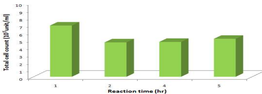
그림 51. Effect of different reaction times on total cell counts of the single cell paste in the scale up experiment from 2 kg to 15 kg paste of korean ginseng. The amount of water was added 1.5 times higher than that of chopping ginseng in the paste and then the mixture was reacted with 0.3% of sumyzyme MC for 60 min at 45 temperature.
