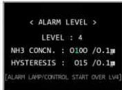
<Fig 4-16> ALARM LEVEL 설정
