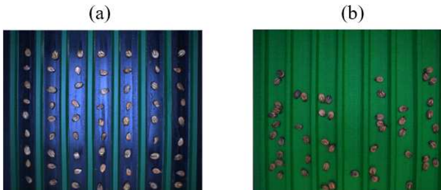
Fig. 27. Conveyor belt modification: (a) original conveyor belt, and (b) modified with green and light absorbing material.
