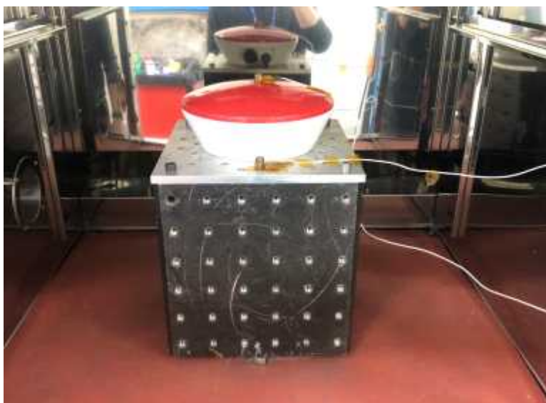
Vibration Test of Embedded Controller Ass'y
