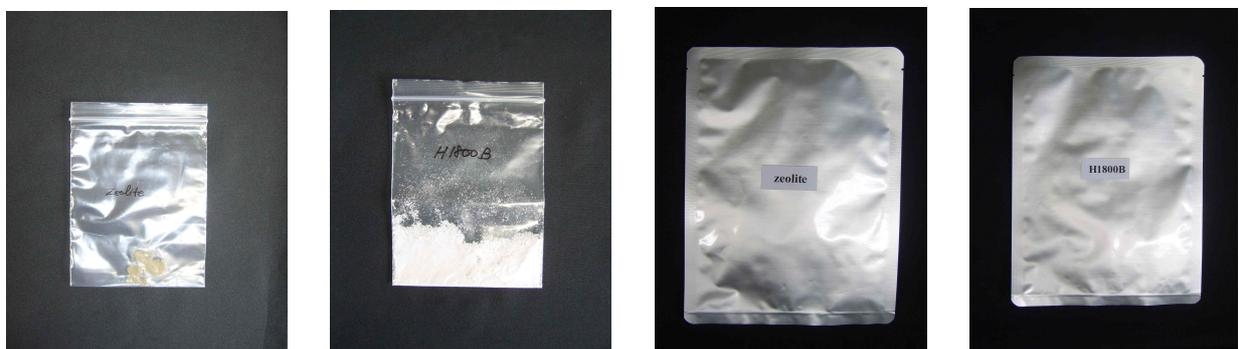
Fig. 1.22. Storage test for a commercial agents. The carrier that microorganism and carrier was mixed in the ratio of one to two was packed and packed it again by one gram. At first, uncolored plastic bag was used and then, colored thick plastic bag was used.
