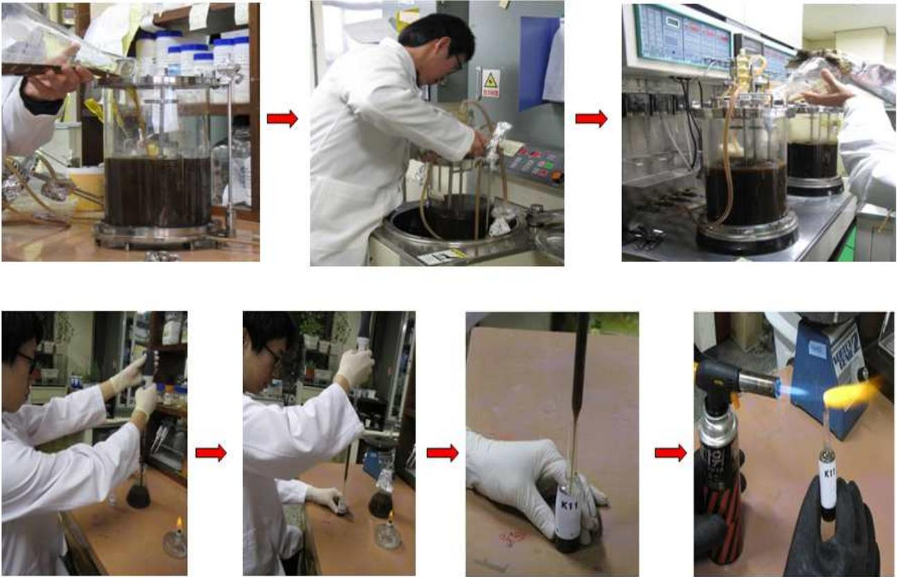
Fig. 1.11. Liquid formulation : Storage test for a commercial agents. Commercial culture of *B. subtilis* AH18, *B. licheniformis* K11 and *P. fluorescens* 2112 for pilot production. Blending of additive materials and packaging of *B. subtilis* AH18, *B. licheniformis* K11 and *P. fluorescens* 2112 for liquid-type pilot production.
